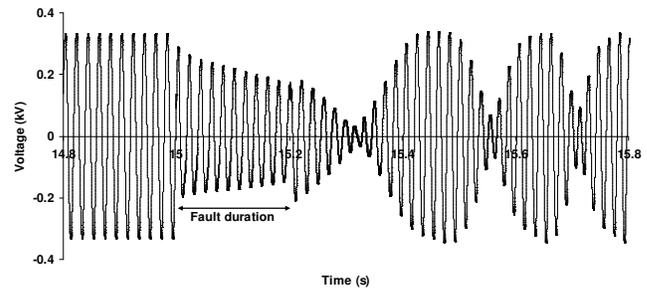
Fig. 11. Generator terminal voltage without the proposed FCL
