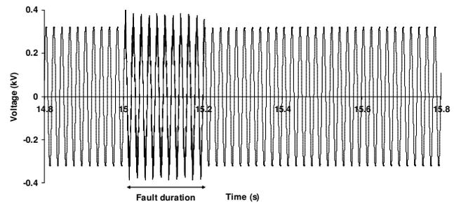
Fig. 12. Generator terminal voltage with the proposed FCL
