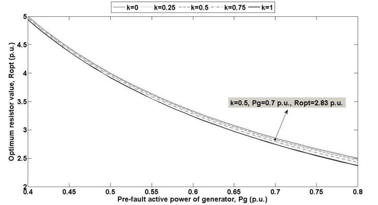
Fig. 6. Optimum resistor variation respect to  $P_g$
