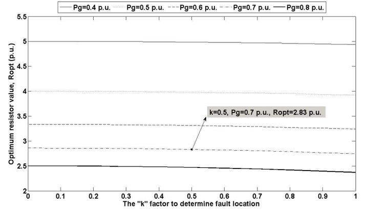
Fig. 5. Optimum resistor variation respect to  $k$
