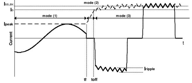
Fig. 2. — — dc reactor current — — Line current (A phase)
