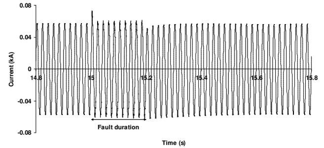
Fig. 10. Generator current with the proposed FCL
