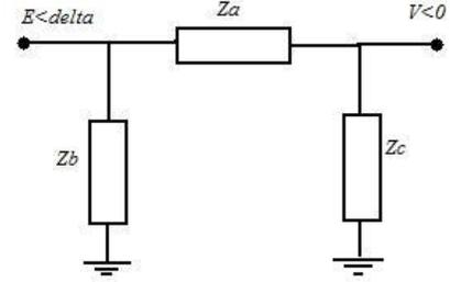
Fig. 4. Equivalent circuit during fault with the proposed FCL
