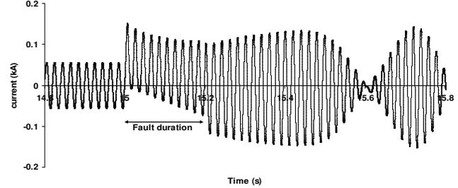
Fig. 9. Generator current without using the proposed FCL
