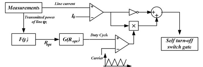
Fig. 7. Control circuit of the proposed FCL
