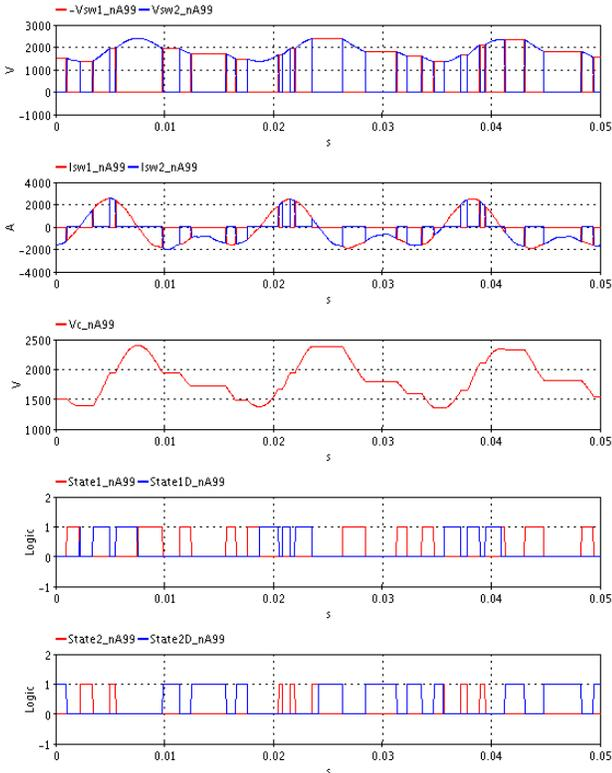
Fig. 8. Switch voltages and currents, capacitor's voltage followed by IGBT and diode states for power module 99 of the lower arm of phase A.
