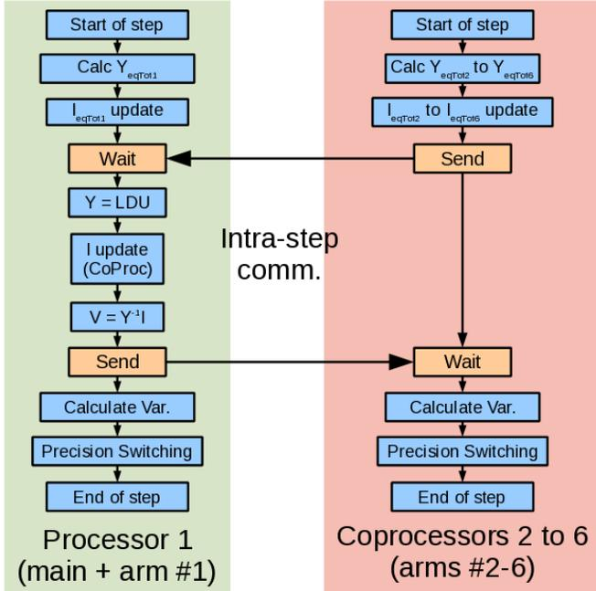
Fig. 7. Converter parallel simulation flowchart for one simulation time step.
