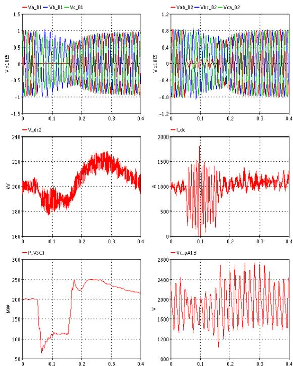
Fig. 13. System waveforms during a single line-to-ground fault on phase A (B1 L-g and B2 L-L voltages, VSC2-side DC bus voltage, DC link current, VSC1 absorbed active power and PM pA13 capacitor voltage).
