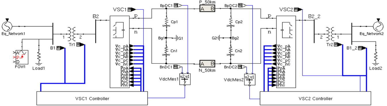
Fig. 10. 225-MVA  $\pm 100$  kV VSC-HVDC 50-km link system.
