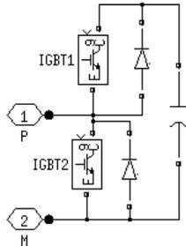
Fig. 2. Power module internal details.
