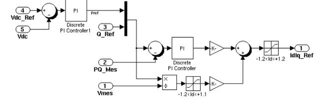
Fig. 5. Basic  $V_{dc}$ -Q controller with feed-forward.
