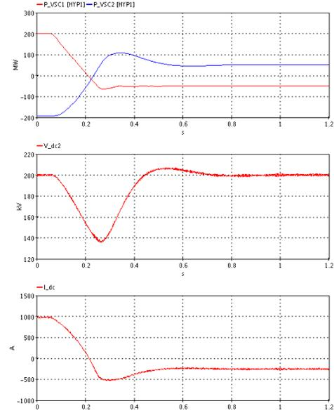
Fig. 11. MMC absorbed power, inverter-side DC voltage and DC current in the 50 km link during a partial power reversal (VSC1 goes from 200 MW to -50 MW in 0.2 s ( $1.25$  GW/s)).
