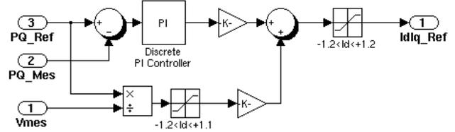
Fig. 4. Basic PQ controller with feed-forward.
