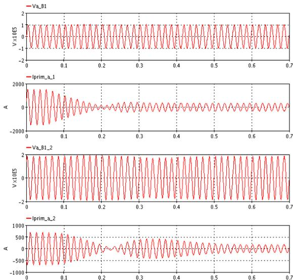
Fig. 12. Voltage of bus B1 and transformer primary currents (phase A only) for both equivalent networks.
