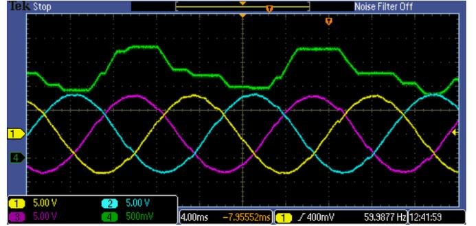
Fig. 9. Screen capture of B2 line-line voltages (scale: 10 kV for 1 V) and capacitor voltage of a power module (scale: 1kV for 1 V).
