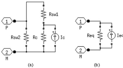
Fig. 6. Power module modeling (a) and equivalent (b).
