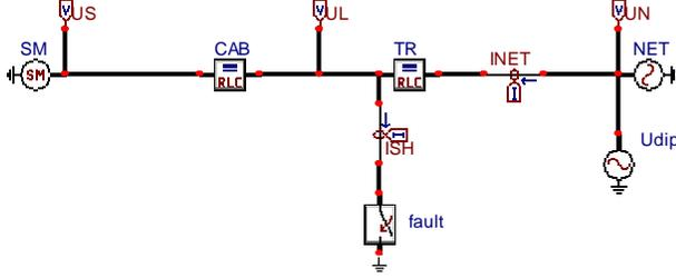
Fig. 2. ATP model of the electrical system
