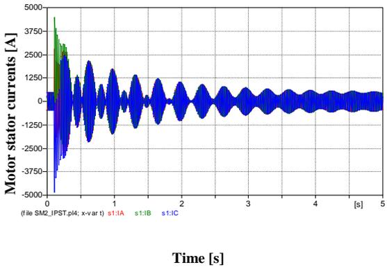
Fig. 8. Stator winding currents as a function of time
