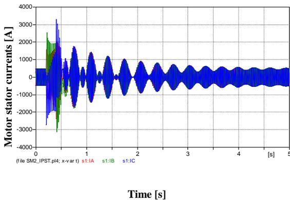
Fig. 12. Stator winding currents as a function of time
