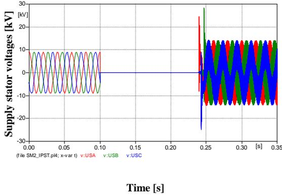
Fig. 3. Stator winding voltages as a function of time (100% dip - 140 ms)
