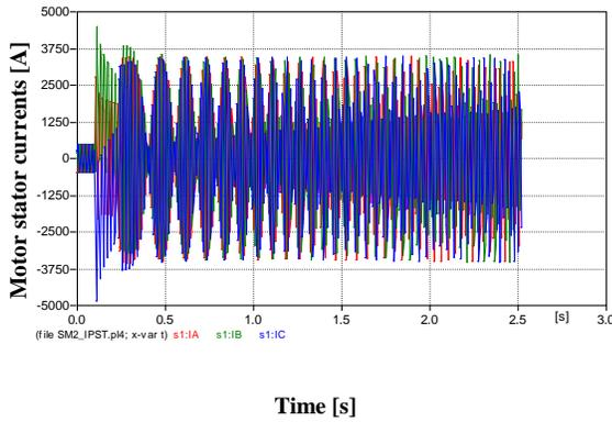
Fig. 4. Stator winding currents as a function of time
