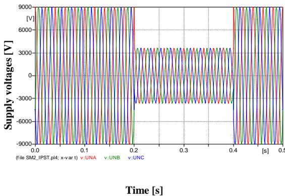
Fig. 11. Voltage dip on network supply voltages as a function of time (60% dip - 200 ms)
