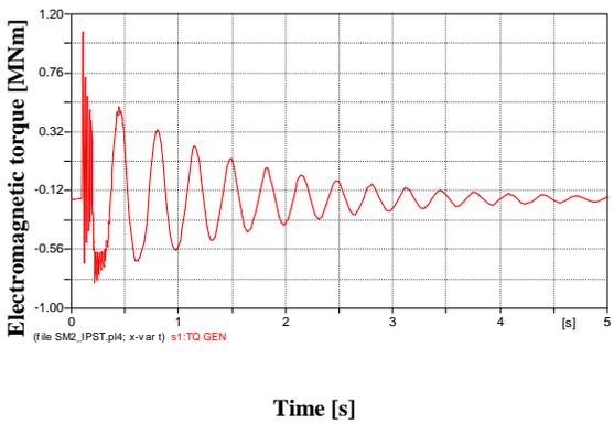
Fig. 9. Electromagnetic torque as a function of time
