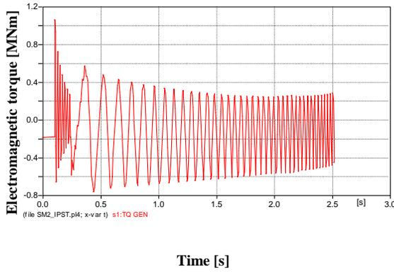
Fig. 5. Electromagnetic torque as a function of time
