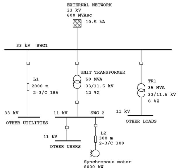
Fig. 1. Single-line diagram of the industrial electrical system
