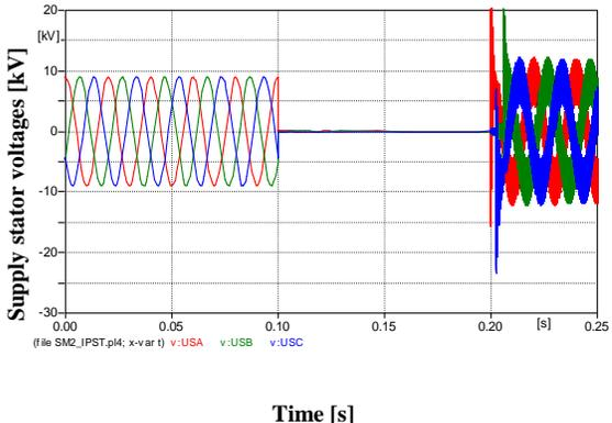
Fig. 7. Stator winding voltages as a function of time (100% dip - 100 ms)
