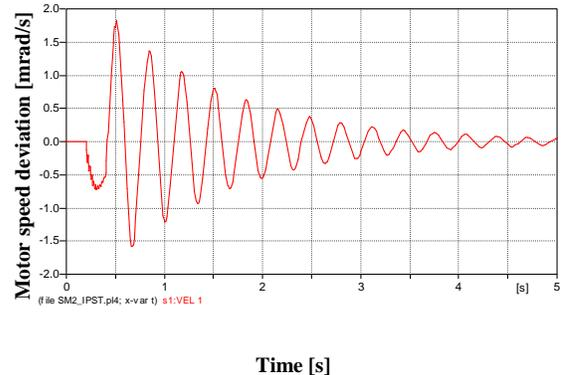
Fig. 14. Angular speed deviation as a function of time
