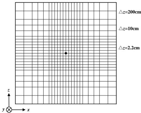
Fig. 2. Cross-sectional ( $zx$ -plane) view of the discretized space around horizontal conductor used in the FDTD computation.
