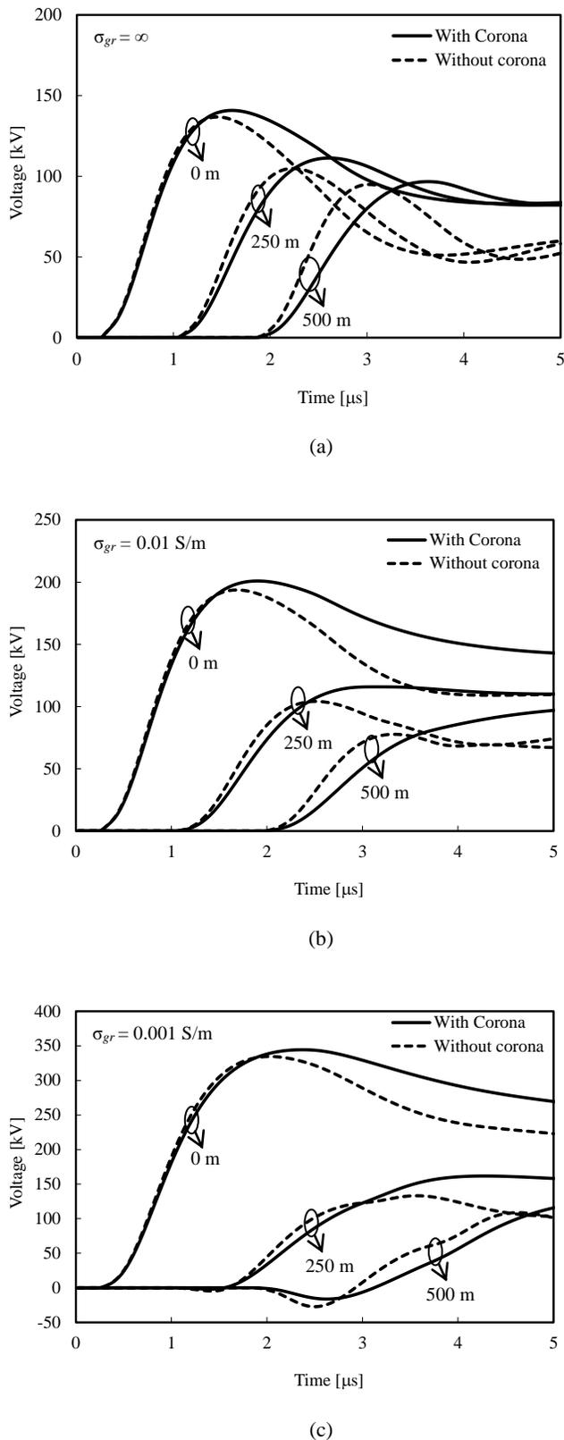
Fig. 5. Stroke location B: FDTD-computed (for  $\sigma_{cor} = 40 \mu\text{S/m}$ ,  $E_0=2.9 \text{ MV/m}$ , and  $E_{cn}=1.5 \text{ MV/m}$ ) waveforms of induced voltages at  $d=0, 250$ , and  $500 \text{ m}$  from the near end of the 5-mm radius, 1-km-long horizontal wire. The computations were performed for (a) perfectly conducting ground ( $\sigma_{gr} = \infty$ ), (b)  $\sigma_{gr} = 0.01 \text{ S/m}$ , and (c)  $\sigma_{gr} = 0.001 \text{ S/m}$ .
