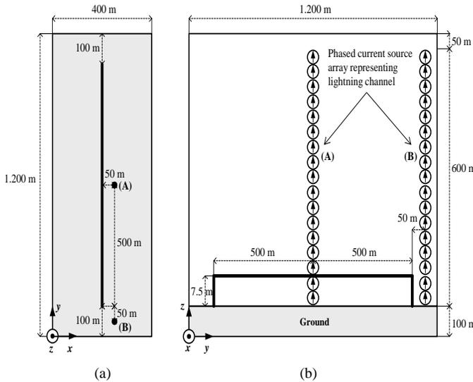
Fig. 1. (a) Plan ( $xy$  plane) and (b) side views ( $yz$  plane) of 5-mm radius, 1-km long overhead horizontal wire located 7.5 m above ground. Corona discharge is assumed to occur only on the horizontal wire.
