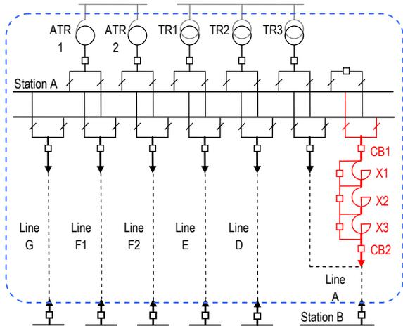
Fig. 2. Single line diagram of the detailed model implemented in EMTP; the model external boundary is evidenced by the dashed blue line.
