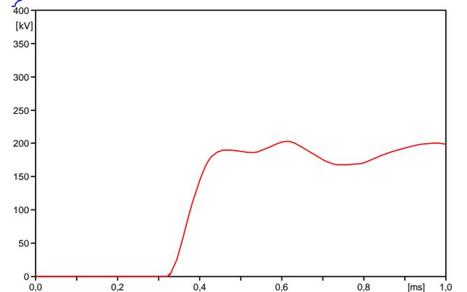
Fig. 5: Fault at CB1 terminals – Network configuration 3 (max short-circuit current).
