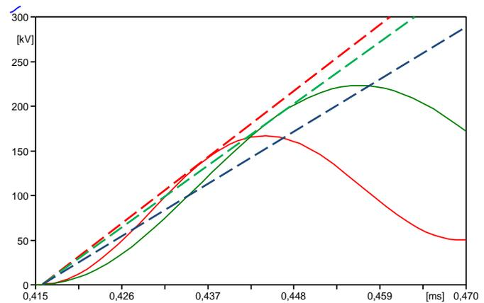
Fig. 10: TRVs for three different series reactors connected.
