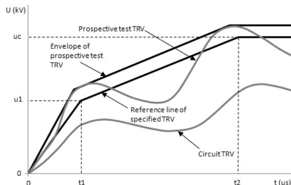
Fig. 1. Example Specified TRV, prospective test TRV and circuit TRV.
