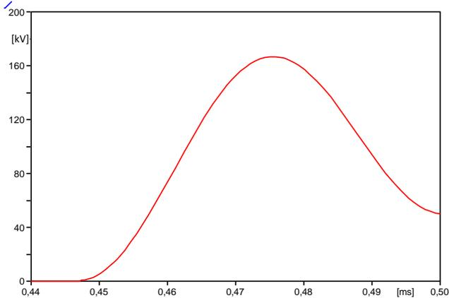
Fig. 7: CB1 TRV - fault at X1 reactor terminals – Network configuration III (max short-circuit current).
