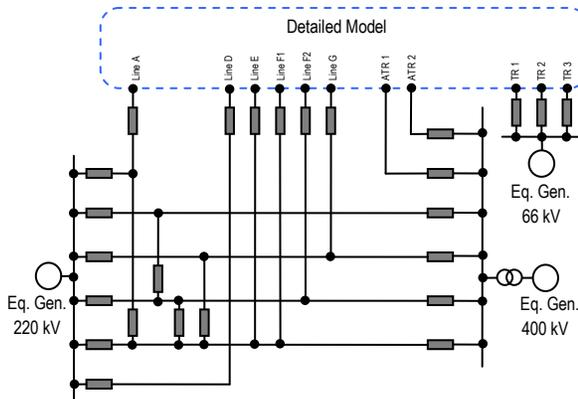
Fig. 3. Short circuit equivalent network model connected to the external boundary of the detailed model
