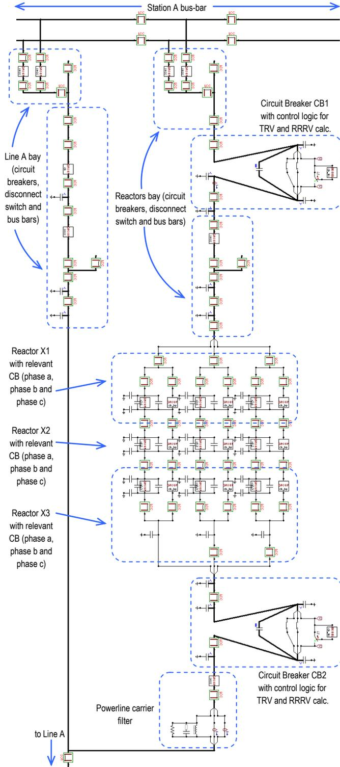
Fig. 4: Power-flow control device portion of the EMTF model.
