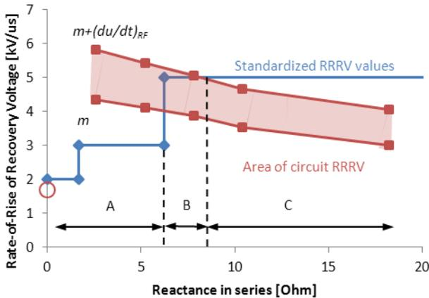
Fig. 11: Simplified method for RRRV compliance verification.
