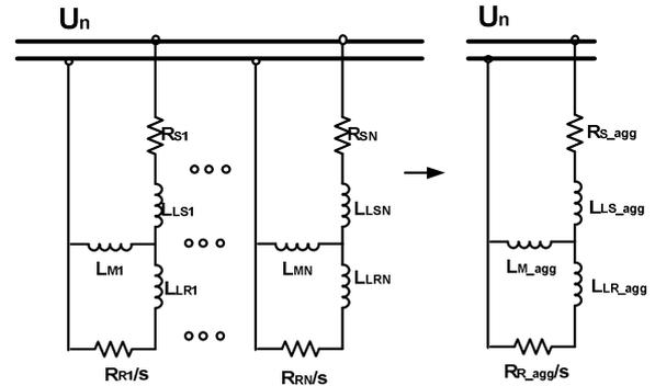
Fig. 8. Aggregation method
