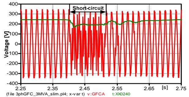
Fig. 17. Behaviour of GFC Output Voltage due to onboard short-circuit
