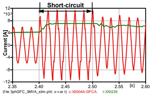
Fig. 19. GFC output current
