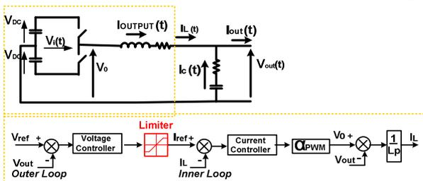
Fig. 4. Control block diagram of the single-phase inverter system
