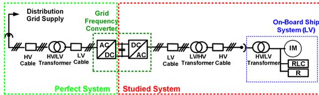
Fig. 3. Shore Connection Distribution Grid topology
