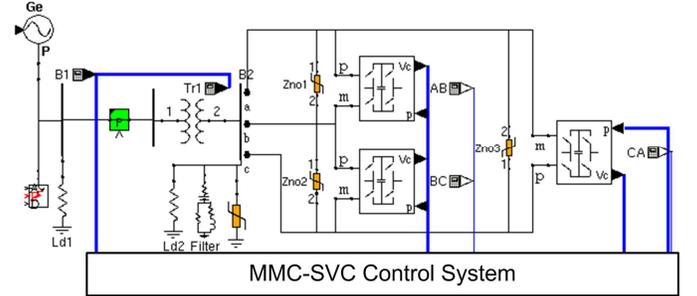
Fig. 6 “Real-time commissioning-ready” modeling of an MMC-STATCOM with a network equivalent at the PCC.
