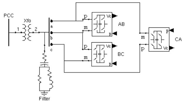
Fig. 1 MMC-SVC delta topology with filters.
