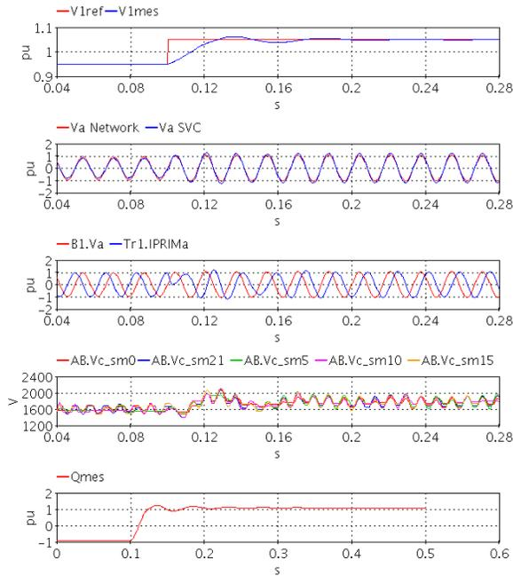
Fig. 7 MMC-SVC waveforms for positive-sequence voltage reference step at 0.1 s: positive-sequence voltage reference and measurement (top), network and SVC voltage (second from top), network voltage and transformer primary current (middle), sample of capacitor voltages from branch AB (second from bottom) and measured reactive power (bottom).
