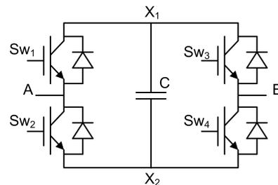
Fig. 2 Power module internal components.
