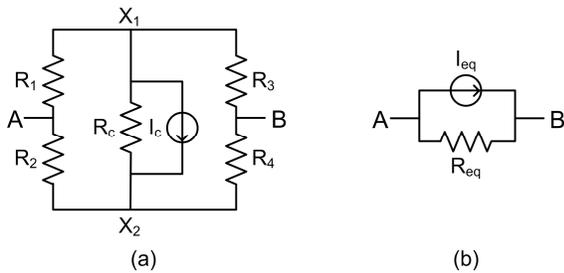
Fig. 3. Power module modeling (a) and equivalent (b).
