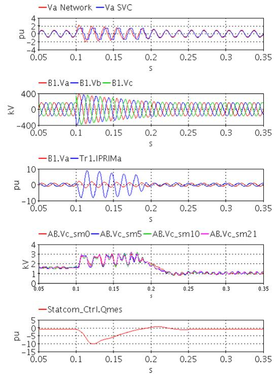
Fig. 8 MMC-SVC waveforms for a network voltage step at 0.1 s: network and SVC voltage (top), transformer primary voltage (second from top), network voltage and transformer primary current (middle), sample of capacitor voltages from branch AB (second from bottom) and measured reactive power (bottom).
