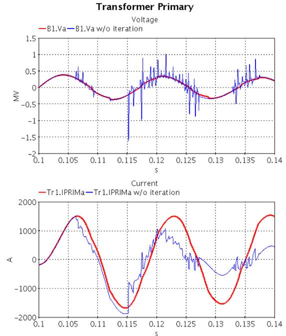
Fig. 9 Comparison of transformer primary voltage and current of phase A during the voltage step with and without iteration (red and blue waveforms respectively).
