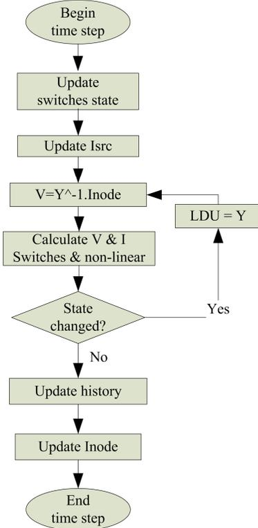
Fig. 4 Iterative engine flowchart.
