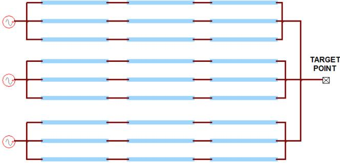
Fig. 2. Simple generic power system with  $N_{gen}=3$  and  $N_{lines}=3$
