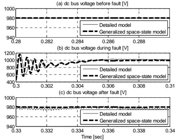
Fig. 13. DC bus voltage before, during and after a dc fault.
