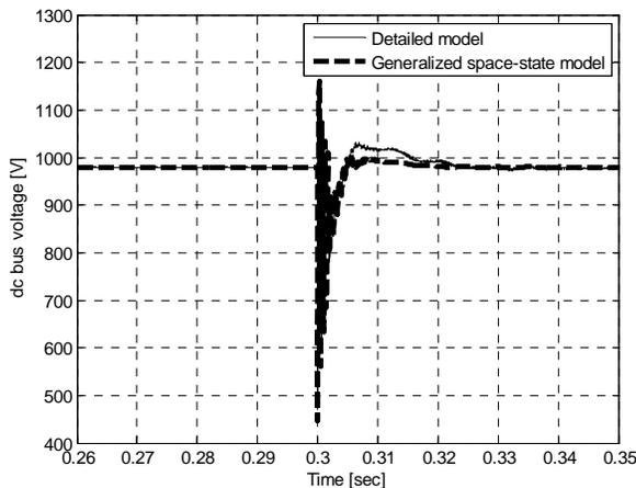
Fig. 12. Transient response of the dc bus voltage due to a dc fault.
