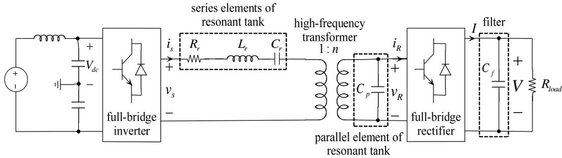
Fig. 2. Resonant circuit under consideration.
