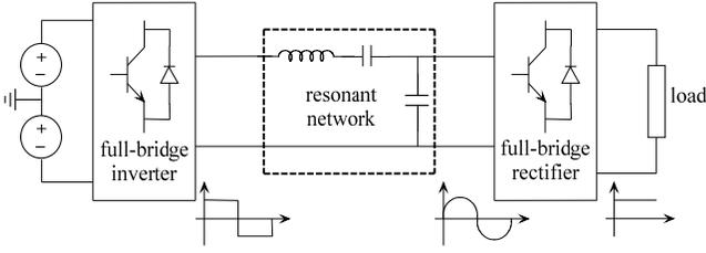
Fig. 1. Simplified circuit diagram of a resonant converter.
