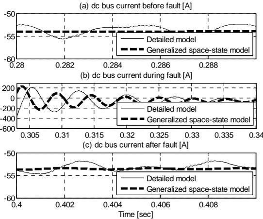
Fig. 11. DC bus current before, during and after a dc fault.
