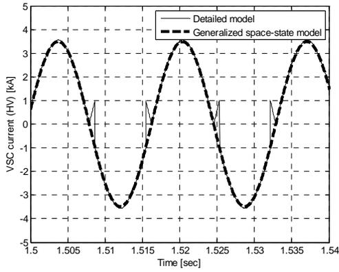
Fig. 4. Comparison of the VSC current (HV).
