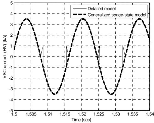
Fig. 4. Comparison of the VSC current (HV).
