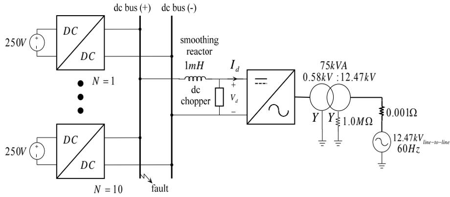
Fig. 3. A dc plant connected to a 60Hz grid through a VSC.
