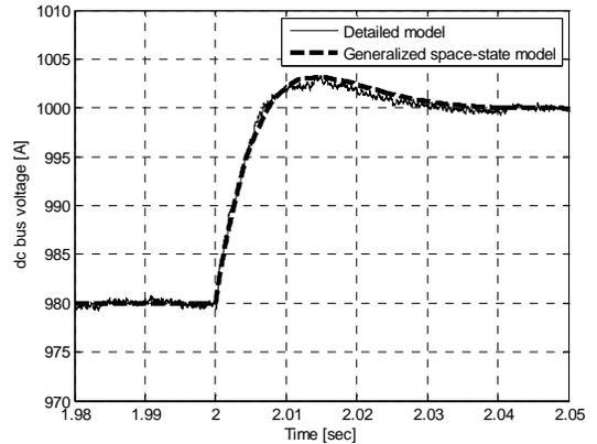
Fig. 9. Transient response comparison of dc bus voltage.
