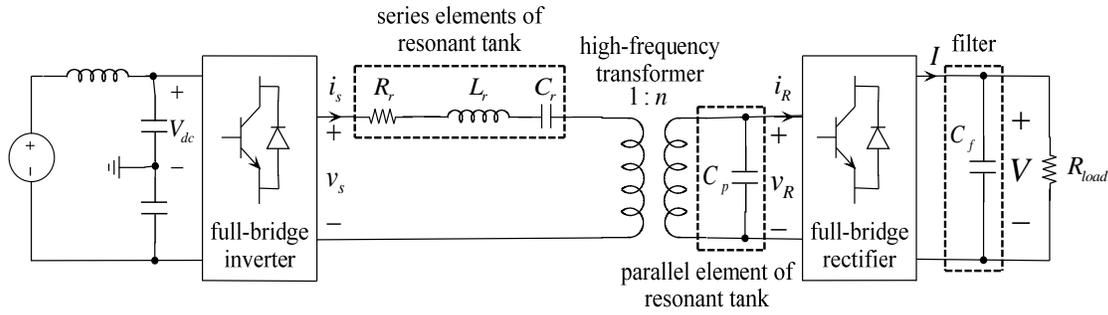
Fig. 2. Resonant circuit under consideration.
