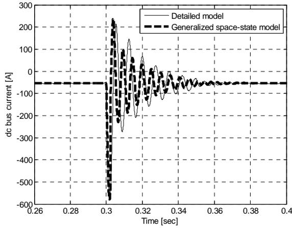
Fig. 10. Transient response comparison of dc bus current due to a dc fault.
