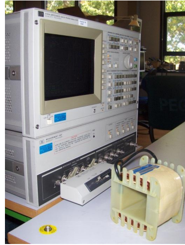
Fig. 2. L-system connection during frequency domain measurements with HP 4149A
