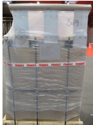
Fig. 8. 4.5 MVar reactor with plastic protection.
