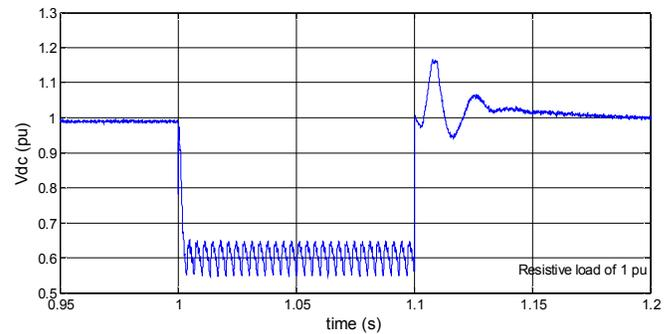
Fig. 7. Blocked state applied in Station#1 for all phase.
