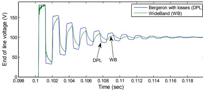
Fig. 5. Open-ended energization test of cable for DPL and WB line models.
