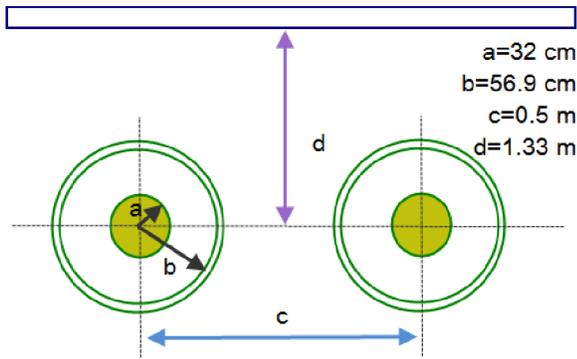
Fig. 4. Cable configuration
