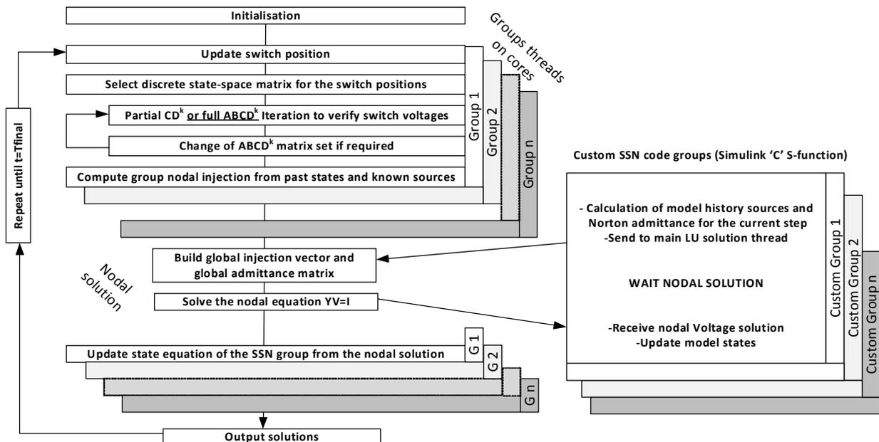
Fig. 1. Simulink implementation of the SSN algorithm with external models
