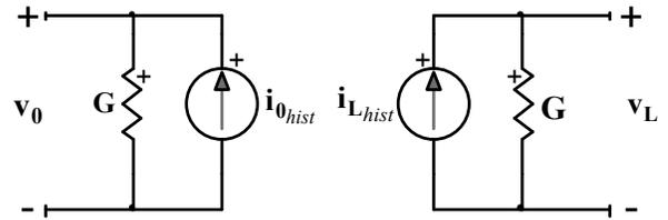
Fig. 3. Reduced discrete time domain circuit of a multi-conductor line
