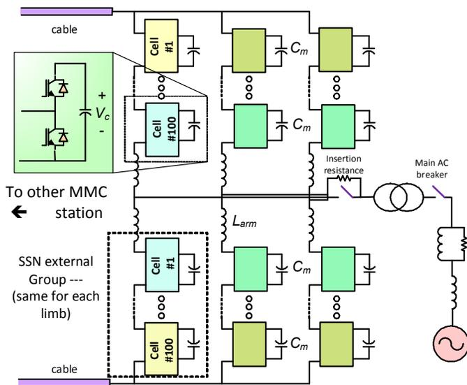
Fig. 6. One MMC-HVDC terminal model
