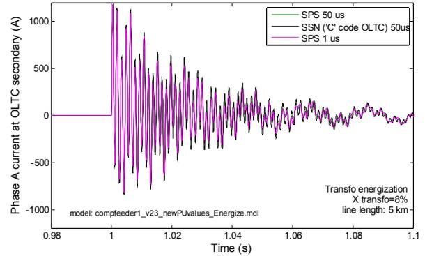
Fig. 10. Distribution grid energization currents (phase A)
