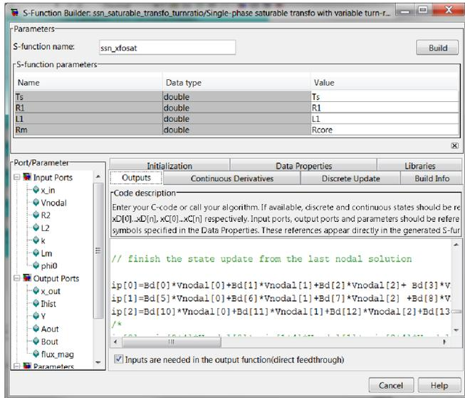
Fig. 2. Simulink S-function builder interface
