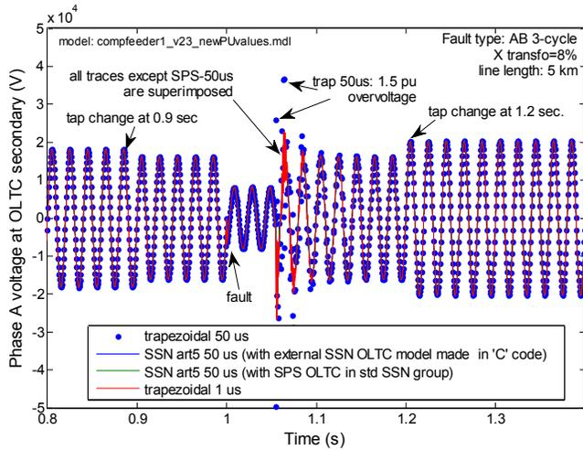
Fig. 9. Comparison between SSN, SSN external model and SPS for two tap changes and phase-phase fault.
