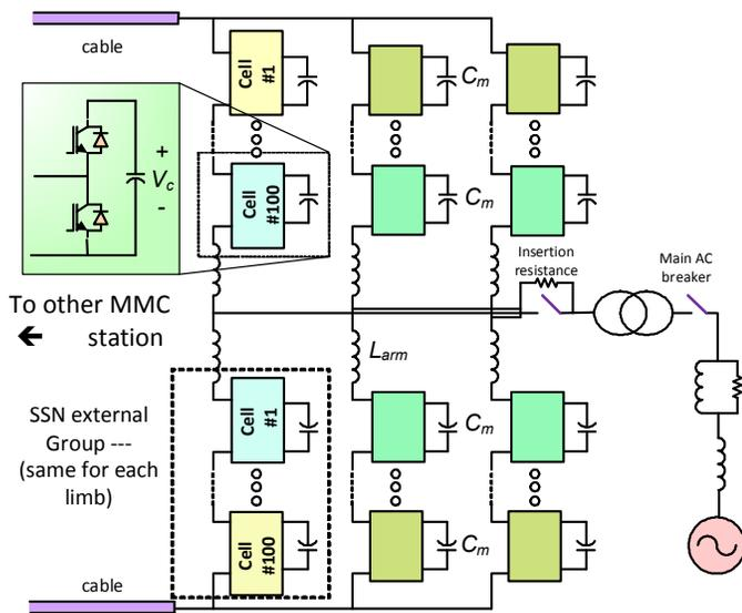
Fig. 6. One MMC-HVDC terminal model
