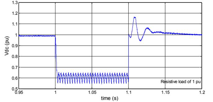
Fig. 7. Blocked state applied in Station#1 for all phase.
