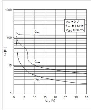
Figure 7: The non-linear capacitance-voltage characteristic of an IGBT [8]
