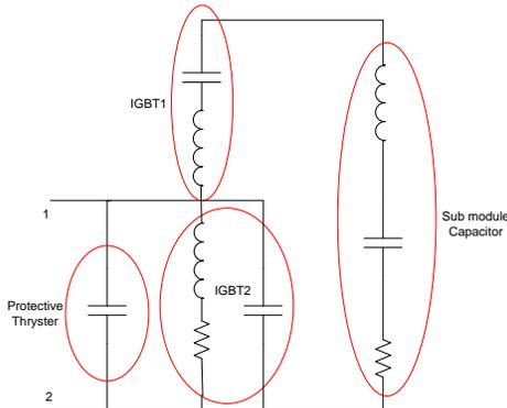
Figure 5: Submodule being turned off implemented in PSCAD
