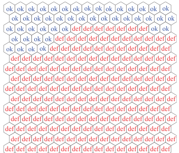
Fig. 6 Operation condition classifier after the training phase.
