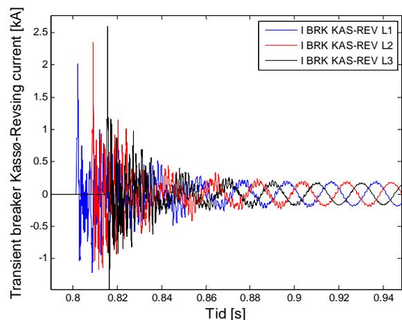
Fig. 13 Breaker current in the breaker Kasso – Revsing, #3 from Fig. 10.
