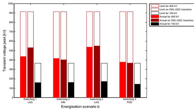
Fig. 7 Results for the second energization scenario of Case Study I, with 4 circuit breakers.
