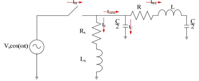
Fig. 2 Single line diagram of the shunt reactor and cable (represented by a single PI).
