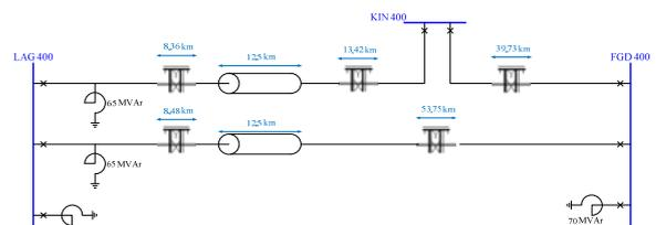
Fig. 4 The Lillebaelt connection for case study I. This line is a combination of OHL and UGC, where the circuit breakers are placed at the substations LAG400, KIN400 and FGD400. Each of these substations also has a 150 kV voltage connection.
