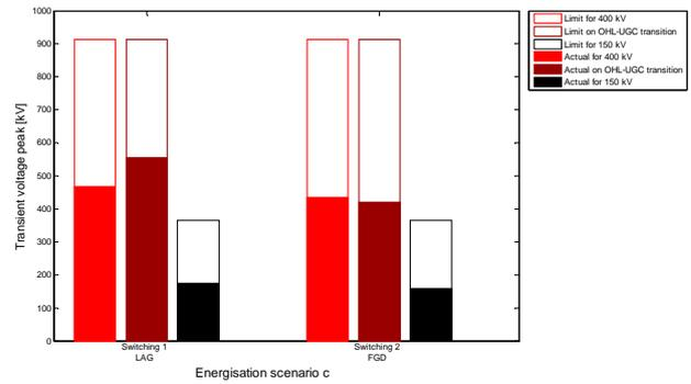
Fig. 8 Results for the third energization scenario of Case Study I, with only 2 circuit breakers.
