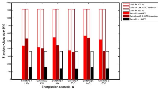
Fig. 6 Results for the first energization scenario of Case Study I, with all 6 circuit breakers.
