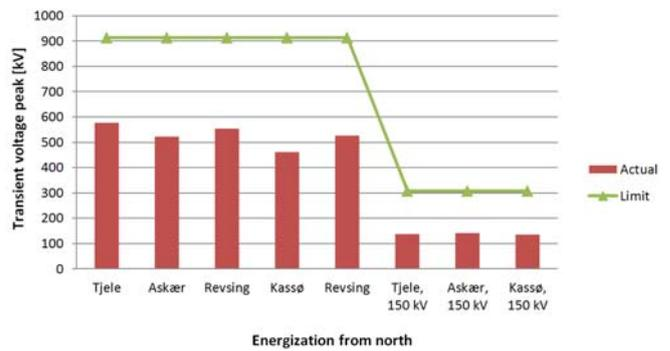
Fig. 12 Results for busbar voltages, for the energization sequence from north of Case Study II.
