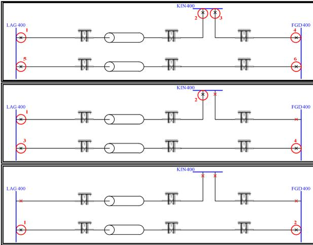
Fig. 5 Possible energization scenarios for the Lillebaelt line of study case I. The switching sequence is shown with circles and numbers
