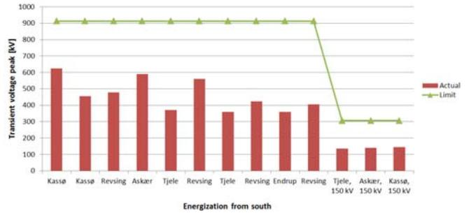
Fig. 11 Results for busbar voltages, for the energization sequence from south from south of Case Study II.
