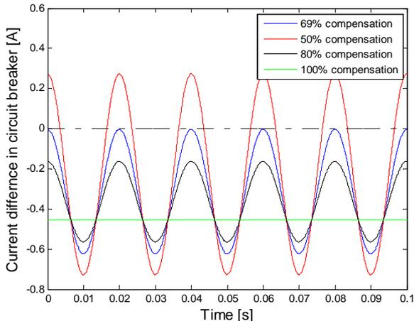
Fig. 3 Breaker current for energization in voltage maximum +1.5 ms, for different levels of compensation.
