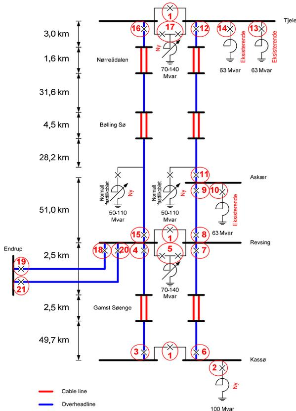
Fig. 10 The Kasso-Tjele connection for case study II. This line is a combination of a double OHL and 2 times double UGC. Each substation also has a 150 kV voltage connection.
