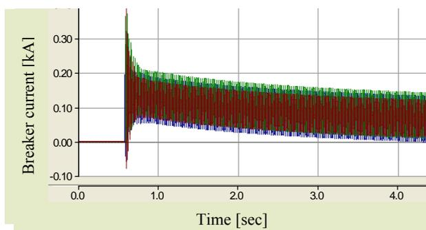
Fig. 1 Line breaker current during energization of a 80% compensated 400 kV cable line. The breaker cannot be re-opened until 4.5 sec after cable energization.
