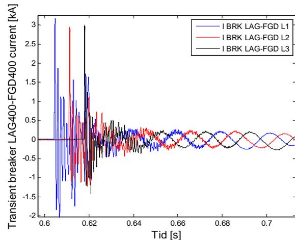
Fig. 9 Breaker current in the breaker LAG400-FGD400 from Fig. 5.
