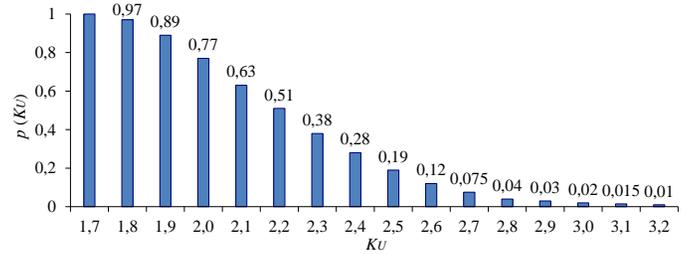
Fig. 1. Estimation of probability for overvoltage generation at arcing ground faults in a distribution network
