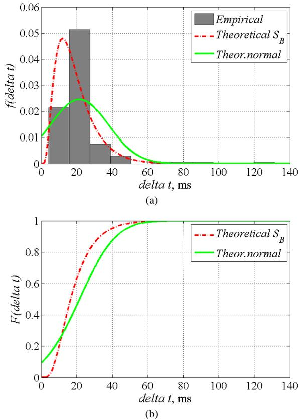
Fig. 6. Density (a) and distribution (b) functions of the Johnson distribution  $S_B$  for the duration of no-current period  $\Delta t$  sample
