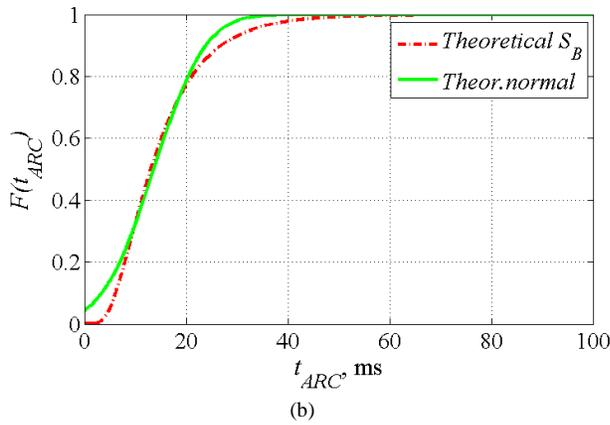
Fig. 5. Density (a) and distribution (b) functions of the Johnson distribution  $S_B$  for the arc duration  $t_{ARC}$  sample
