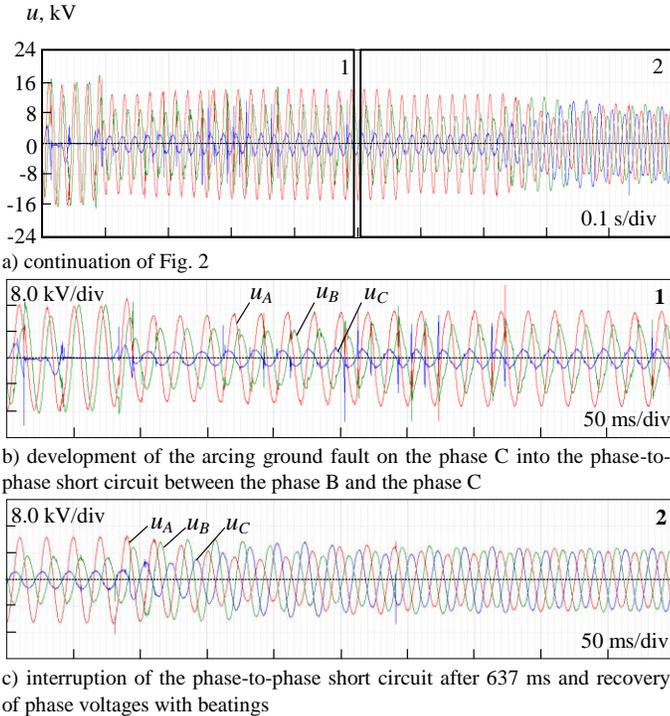
Fig. 3. Real oscillogram of development of the arcing ground fault into the phase-to-phase short circuit in the MIPI cable in the 10 kV network (ending of the fault)
