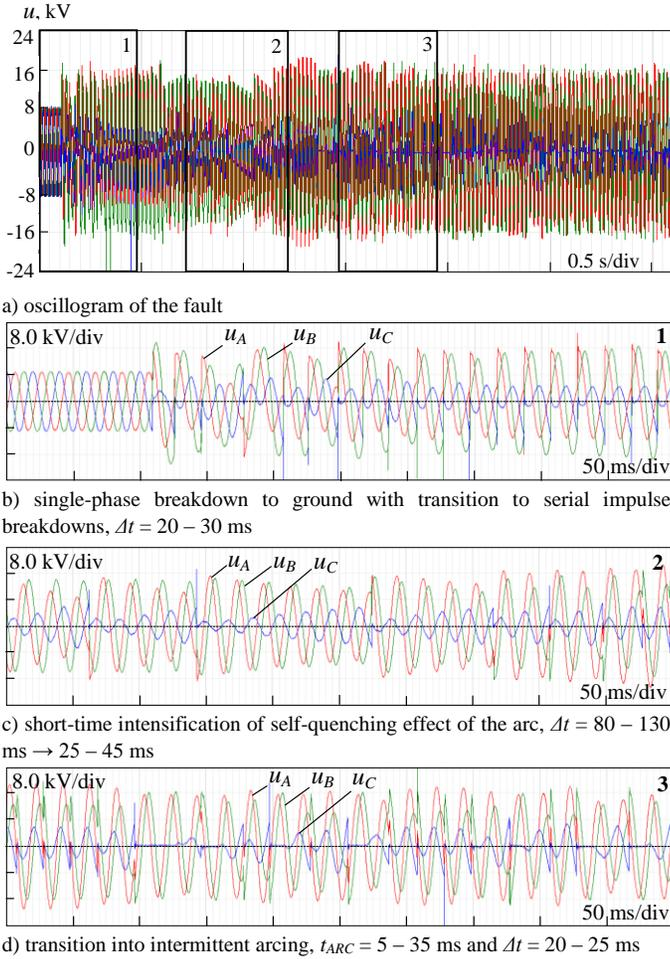
Fig. 2. Real oscillogram of the arcing ground fault in the MIPI cable in the 10 kV network (beginning of the fault)
