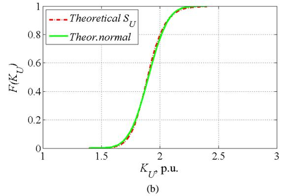
Fig. 7. Density (a) and distribution (b) functions of the Johnson distribution  $S_U$  for the overvoltage level  $K_U$  sample
