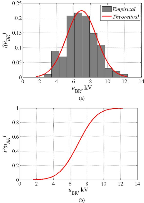
Fig. 4. Density function (a) and distribution function (b) for the breakdown voltage  $u_{BR}$  sample
