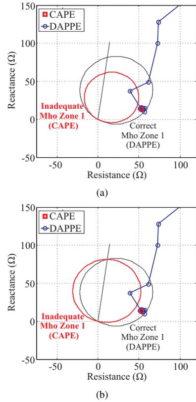
Fig. 11. Three-phase fault simulations using relays incorrectly set: (a) Zone 1 with 60% instead of 80%, (b) Torque angle equal to 75° instead of 60°.
