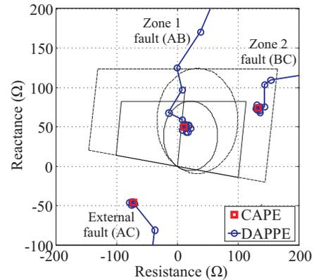
Fig. 8. Line-to-line fault simulations.
