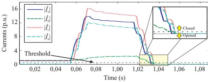
Fig. 4. CB opening detection procedure.
