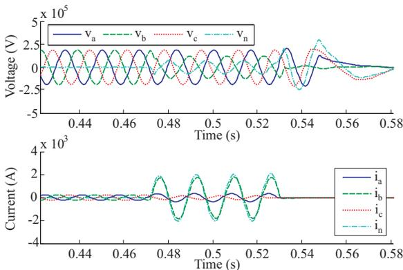
Fig. 13. Voltage and current records taken from the substation CCD.
