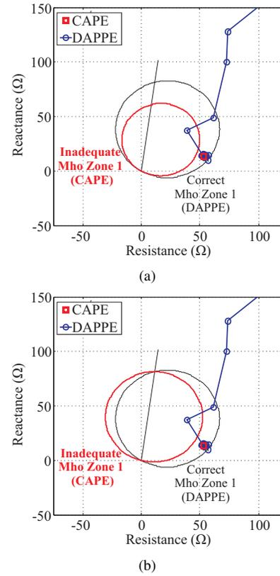
Fig. 11. Three-phase fault simulations using relays incorrectly set: (a) Zone 1 with 60% instead of 80%, (b) Torque angle equal to  $75^\circ$  instead of  $60^\circ$ .
