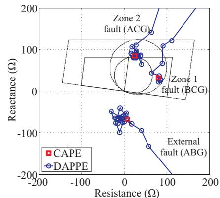
Fig. 9. Double-line-to-ground fault simulations.
