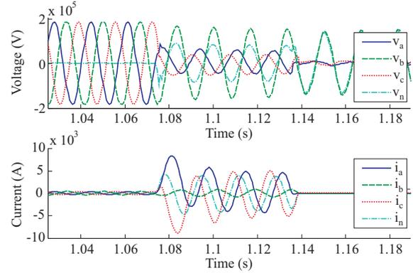
Fig. 14. Voltage and current records taken from the substation GNN.
