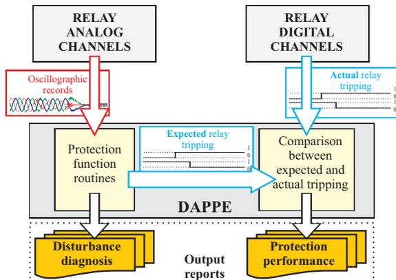
Fig. 1. DAPPE block diagram.
