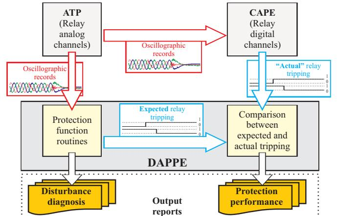
Fig. 5. DAPPE block diagram for disturbance analysis using ATP and CAPE.
