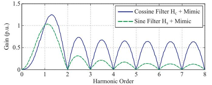
Fig. 2. Frequency response of the FCDFT+Mimic filters.
