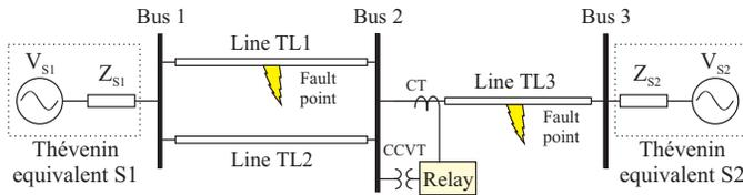
Fig. 6. 230 kV test power system.
