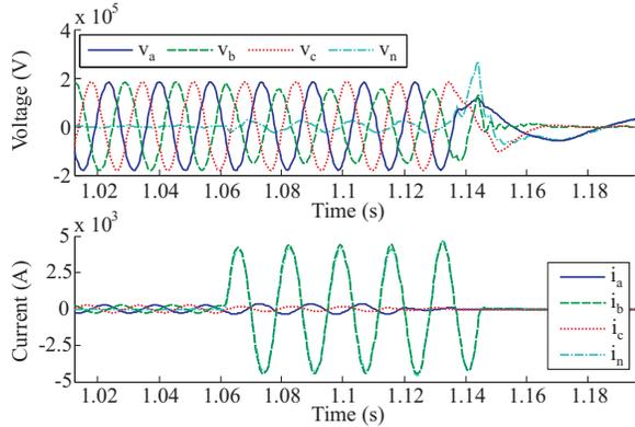
Fig. 12. Voltage and current records taken from the substation PAF.
