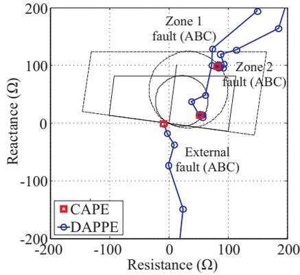
Fig. 10. Three-phase fault simulations.
