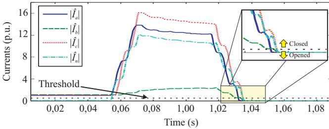
Fig. 4. CB opening detection procedure.
