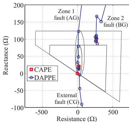
Fig. 7. Single line-to-ground fault simulations.
