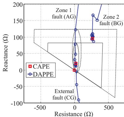
Fig. 7. Single line-to-ground fault simulations.
