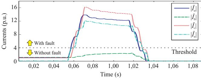
Fig. 3. Fault type classification procedure.
