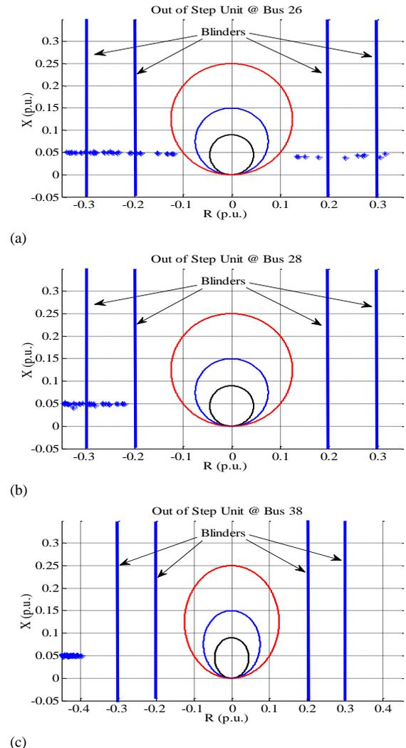
Fig. 8. Out-of-step relays outputs installed at buses 26, 28 and 38 during electromechanical wave propagation
