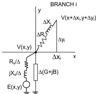
Fig. 1. Incremental system used for continuum modeling of system
