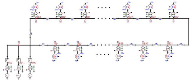
Fig. 2. 64-Generator ring system modeled in ATP
