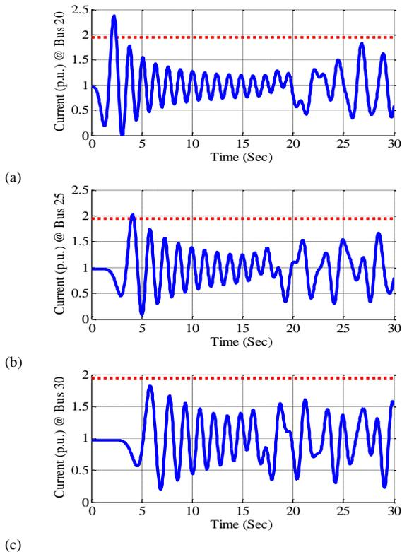
Fig. 6. Outputs of overcurrent relays installed at buses 20, 25 and 30 during electromechanical transient propagation
