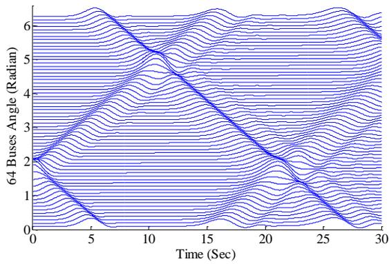
Fig. 3. Electromechanical wave propagation after a disturbance at bus 16
