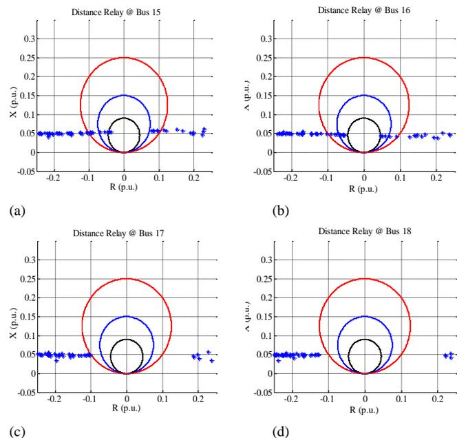
Fig. 7. Distance relays outputs installed at buses 15, 16, 17 and 18 during electromechanical wave propagation
