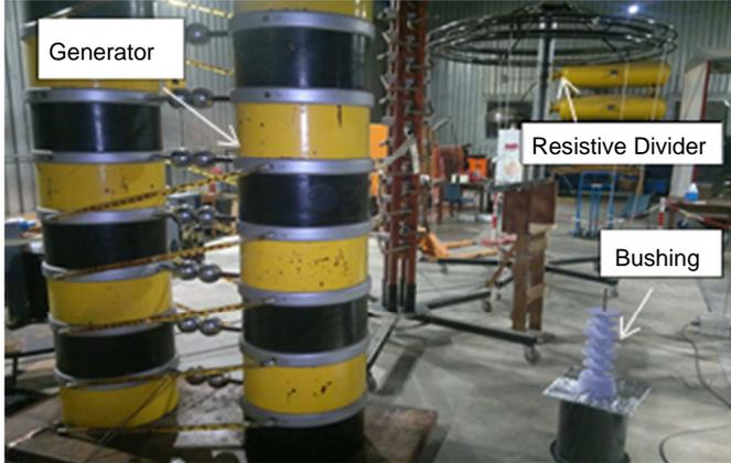
Fig. 7. Impulse voltage measurement setup
