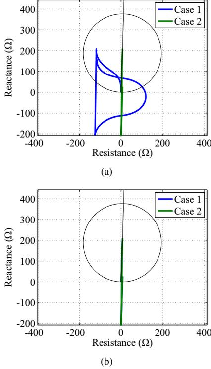
Fig. 9. Apparent impedances calculated by a  $Z_{AG}$  relay unit at Bus N (a) AG and (b) ABC faults along the  $\lambda/2^+$  extension considering 2 formulations: unconventional with  $k_1$  and  $k_2$  calculated for a fault at the end of transmission line (Case 1) and; unconventional with  $k_1$  and  $k_2$  calculated for the exact fault location (Case 2).
