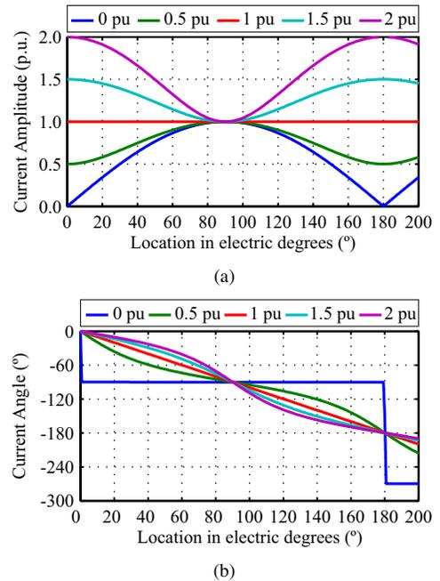
Fig. 2. Current phasor profiles along a  $\lambda/2^+$  for different load flow conditions: (a) amplitude and (b) angle.
