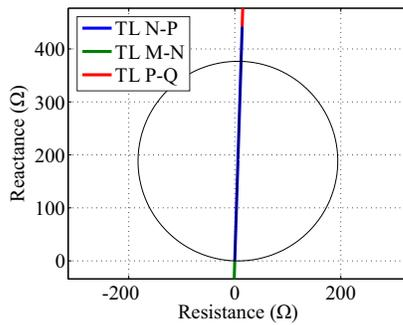
Fig. 12. Apparent impedance calculated by a relay installed at Bus N for any fault type along the three lines extension considering the unconventional distance protection formulation proposed in [15] combined with the correction method proposed in this paper.
