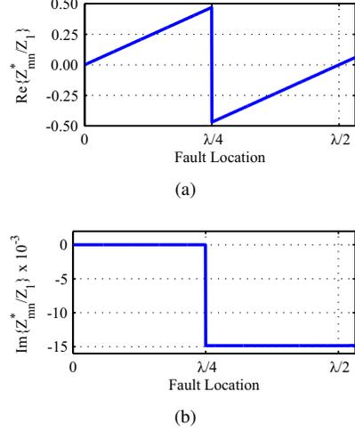
Fig. 11. (a) Real and (b) imaginary parts of the *per unit* corrected apparent impedance.
