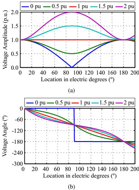
Fig. 1. Voltage phasor profiles along a  $\lambda/2^+$  for different load flow conditions: (a) amplitude and (b) angle.
