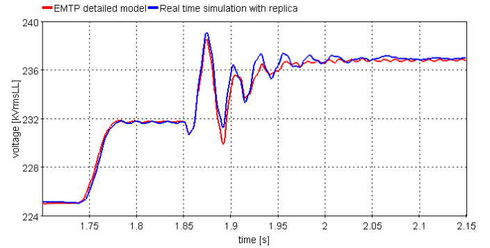
Fig. 4 Domloup SVC voltage response for 13,5 kV sudden variation of the voltage reference; red curve: EMTP detailed model; blue curve: Hypersim simulation connected to SVC study replica
