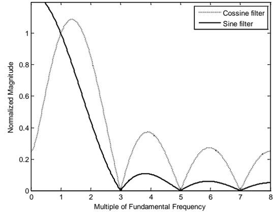
Fig. 3. Magnitude response of the HDFT algorithm.
