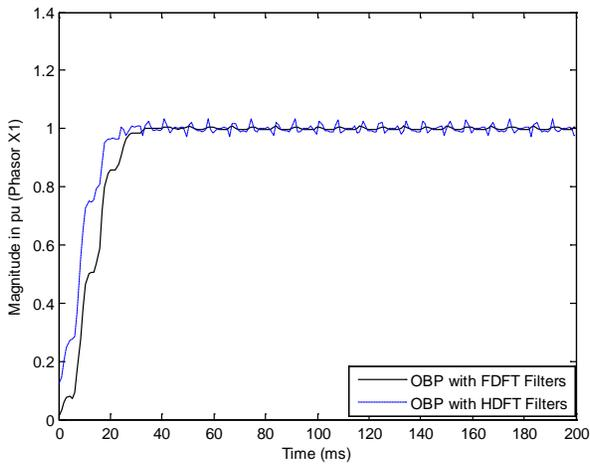
Fig. 15. Fundamental phasor magnitude of the signal  $x_1$  (Proposed technique).
