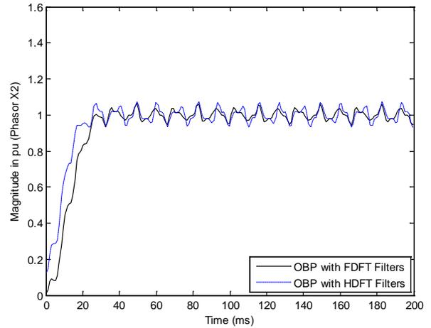
Fig. 17. Fundamental phasor magnitude of the signal  $x_2$  (Proposed technique).
