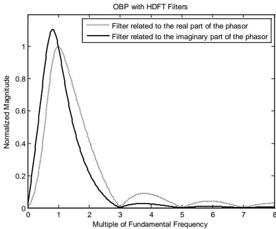
Fig. 8. Magnitude response of the combination: OPB filter with HDFT filters.
