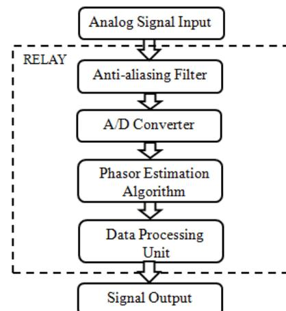
Fig. 1. Basic Relay Architecture Representation.
