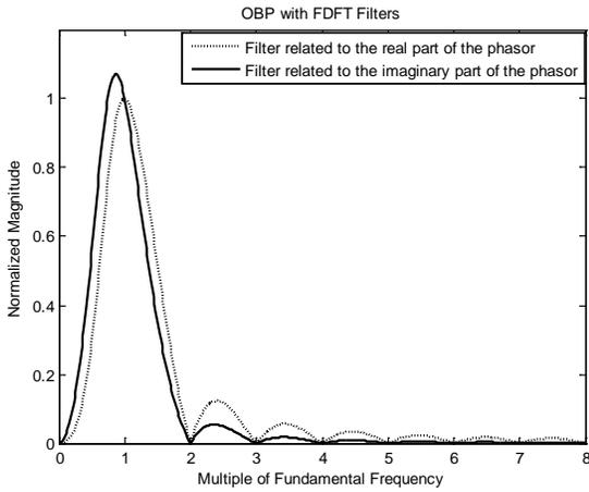
Fig. 7. Magnitude response of the combination: OPB filter with FDFT filters.
