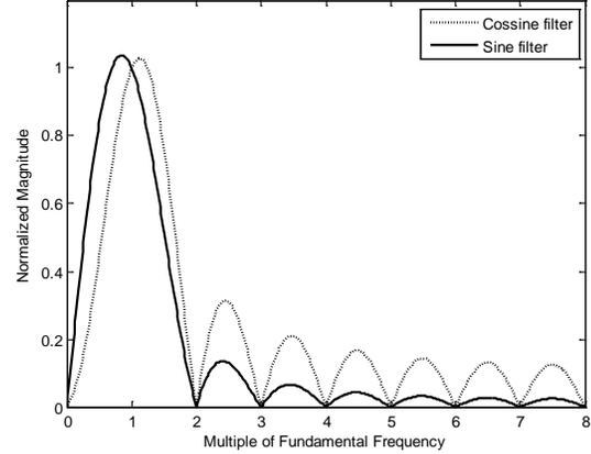
Fig. 2. Magnitude response of the FDFT algorithm.
