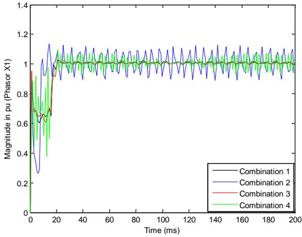
Fig. 14. Fundamental phasor magnitude of the signal  $x_1$  (Classical methods).
