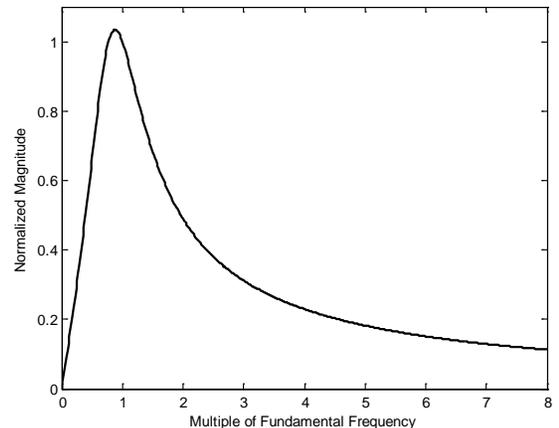
Fig. 5. Magnitude response of the Optimized Band-Pass Filter.
