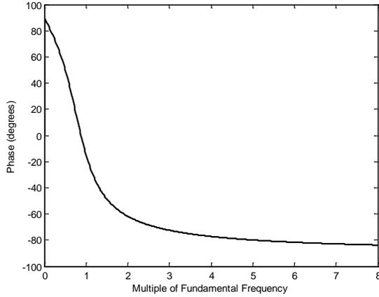
Fig. 6. Phase response of the Optimized Band-Pass Filter.
