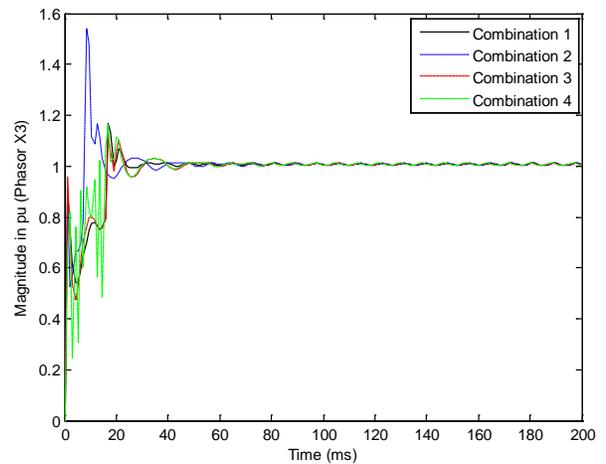
Fig. 18. Fundamental phasor magnitude of the signal  $x_3$  (Classical methods).
