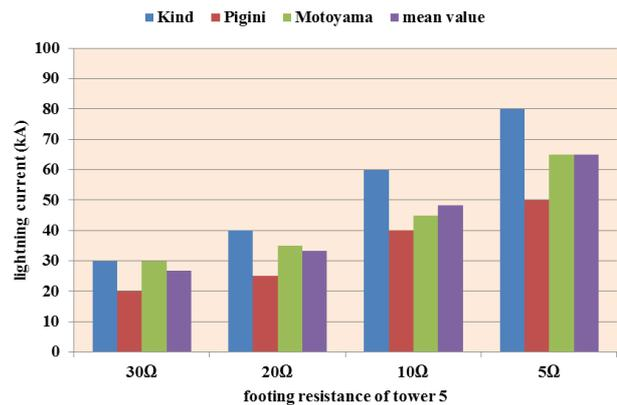
Fig. 14. Minimum lightning peak currents causing backflashover across the insulator string of 110-kV circuit for various values of footing resistance in response to the first stroke on tower top
