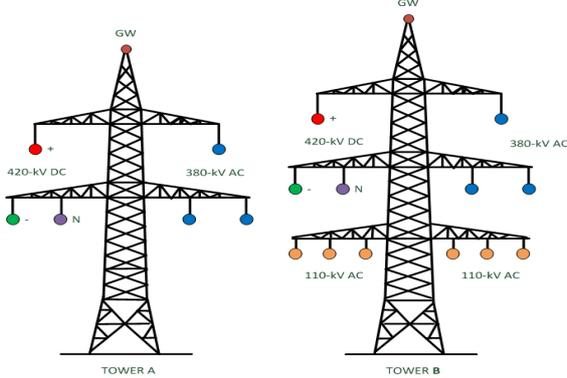
Fig. 1. Layout of multi-circuit suspension towers
