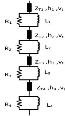
Fig. 2. Tower model with additional  $RL$ -circuits.
