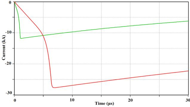
Fig. 3. Lightning current waveform with median values.
