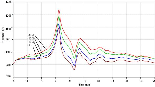
Fig. 4. Overvoltages across the upper insulator string of positive pole for various values of footing resistance in response on first stroke on tower top.
