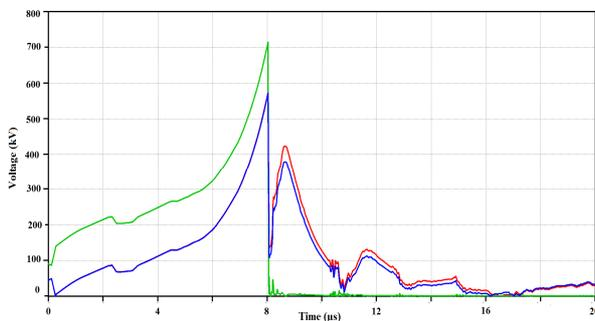
Fig. 12. Overvoltages across the insulator strings of 110-kV conductors for in response to first stroke on tower top.
