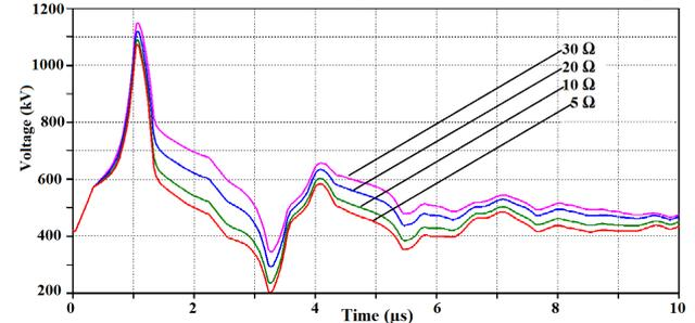
Fig. 11. Overvoltages across the upper insulator string of positive pole for various values of footing resistance in response to subsequent stroke on tower top.
