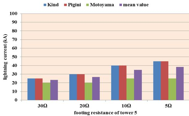
Fig. 15. Minimum lightning peak currents causing backflashover across the insulator string of 110-kV circuit for various values of footing resistance in response to the subsequent stroke on tower top
