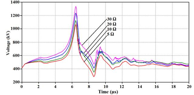
Fig. 10. Overvoltages across the upper insulator string of positive pole for various values of footing resistance in response to first stroke on tower top.
