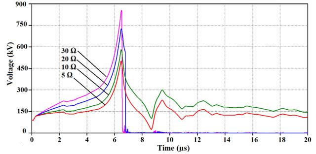
Fig. 8. Overvoltages across the lower insulator string of 110-kV circuit for various values of footing resistance in response to first stroke on tower top.
