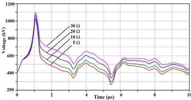
Fig. 5. Overvoltages across the upper insulator string of positive pole for various values of footing resistance in response on subsequent stroke on tower top
