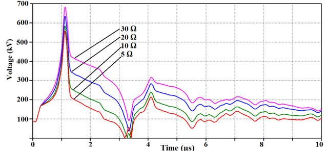
Fig. 9. Overvoltages across the lower insulator string of 110-kV circuit for various values of footing resistance in response to subsequent stroke on tower top.
