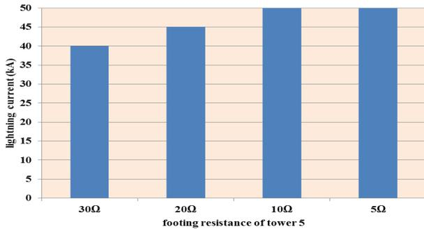
Fig. 7. Minimum lightning currents causing backflashover across the upper insulator string of positive pole for various values of footing resistance in response to subsequent stroke on tower top.
