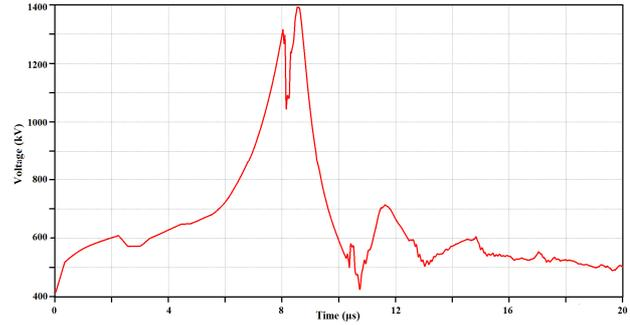
Fig. 13. Overvoltages across the upper insulator string of positive pole for in response to first stroke on tower top.
