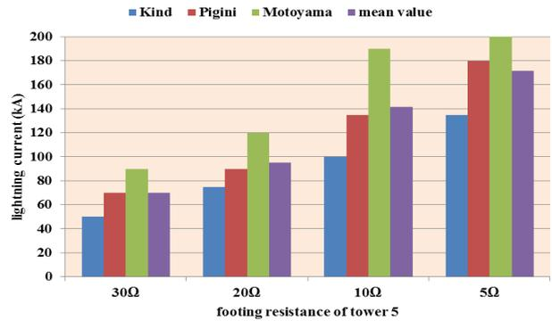
Fig. 6. Minimum lightning current causing backflashover across the upper insulator string of plus pole of HVDC circuit for various values of footing resistance in response on first stroke on tower top
