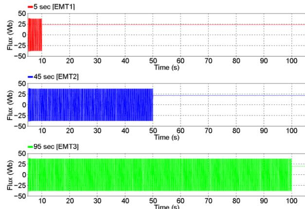
Fig. 19. Variation of residual flux depending on duration time (Top: 5 sec – 23.7 Wb-t, Middle: 45 sec – 22.1 Wb-t, Bottom: 95 sec – 20.2 Wb-t).
