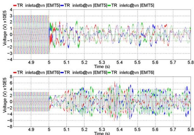
Fig. 11. Voltages at transformer primary side for Case 3 (upper) and Case 4 (lower).
