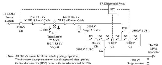
Fig. 1. Single line diagram of 380 kV circuit to 380 / 13.8 kV transformer.
