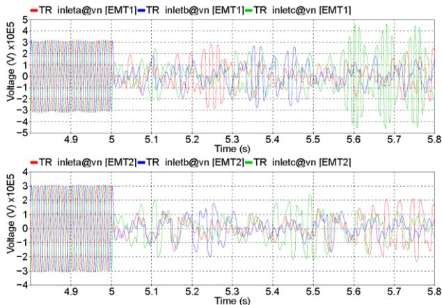
Fig. 7. Voltages at transformer primary side for Case 1 (upper) and Case 2 (lower).
