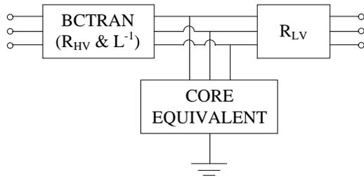
Fig. 3. BCTRAN transformer model with externally attached core [3].
