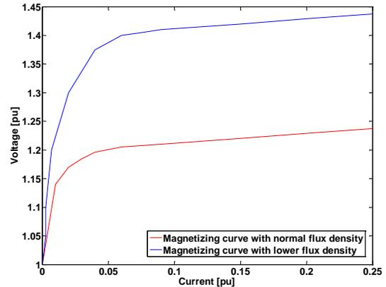
Fig. 8. Magnetizing curve of power transformer
