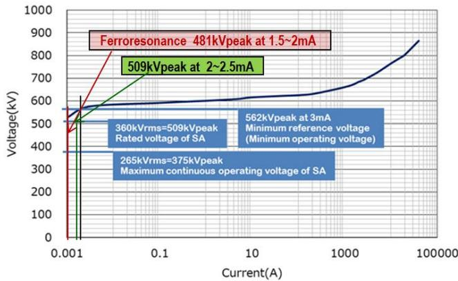
Fig. 17. Typical V-I characteristics of 360 kV surge arrester.
