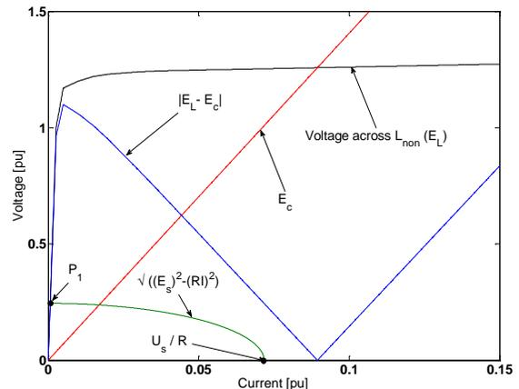
Fig. 13. Graphical solution of series non-linear ferroresonance circuit with resistance [1].
