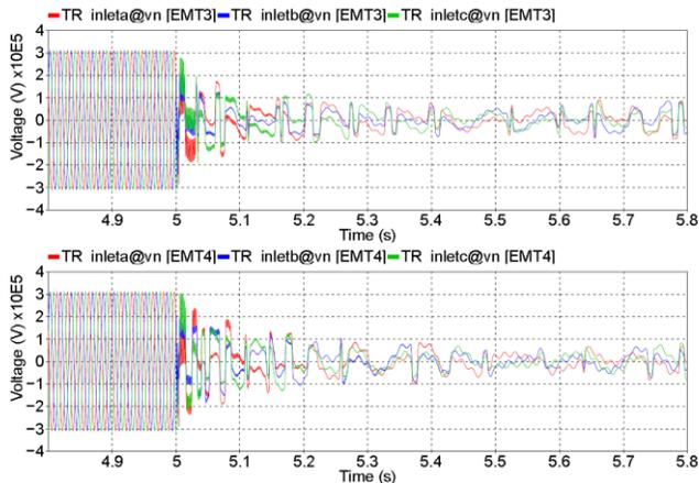
Fig. 10. Voltages at transformer primary side for Case 1 (upper) and Case 2 (lower).
