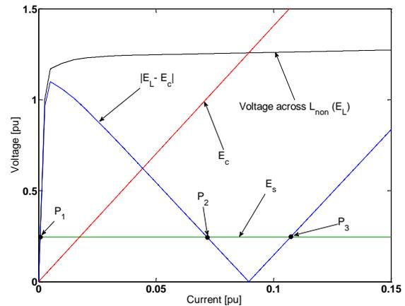
Fig. 12. Graphical solution of series non-linear ferroresonance circuit without resistance [7].
