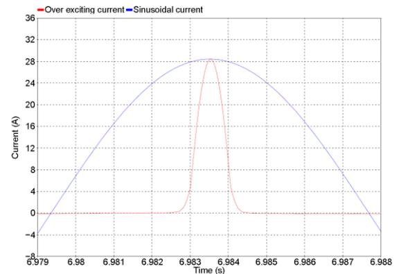
Fig. 16. Enlarged view of over exciting current for basic case together with the sinusoidal current
