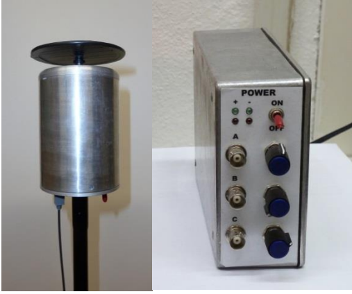
Fig. 2, E-field sensor (left) and 3-channel receiver unit with amplifiers and offset tuning
