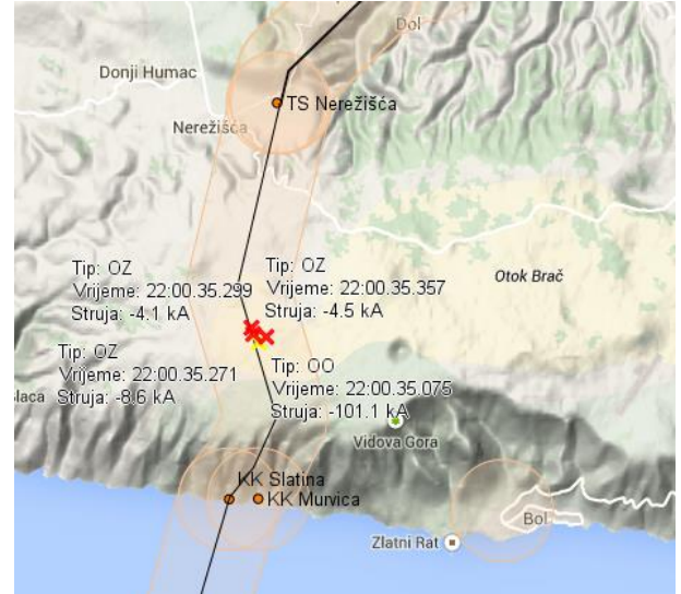
Fig. 6. Time and spatial correlation between relay protection system and LLS data, Case 1
