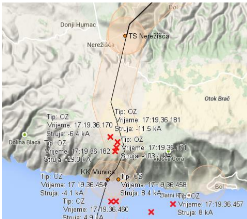
Fig. 9. Time and spatial correlation between relay protection system and LLS data, Case 2
