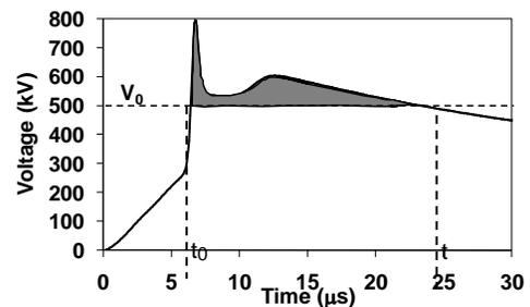
Fig. 4. Stylized representation of the DE method for determining the critical current leading the insulators to backflashover.
