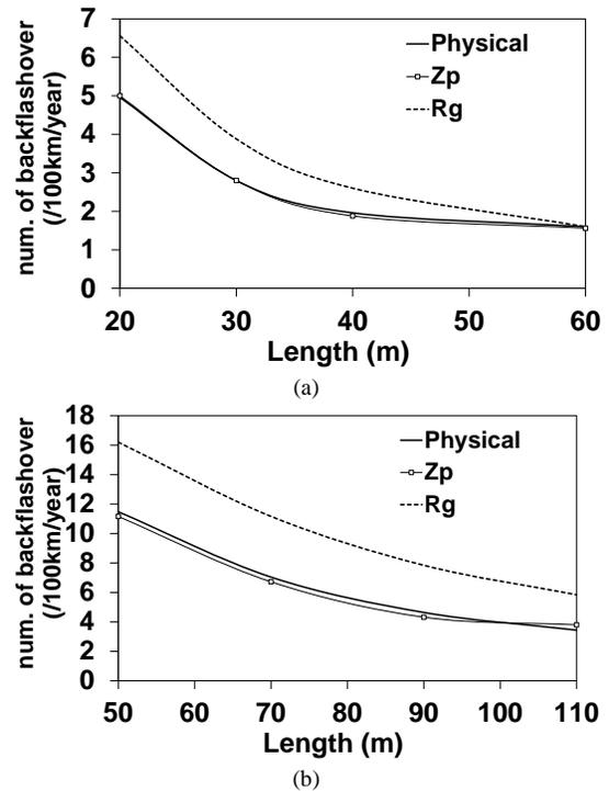
Fig. 5. Comparison of the outages rates calculated from the different representations of the tower-footing electrodes. Soil resistivity of: (a) 600 and (b) 2000  $\Omega$ m.
