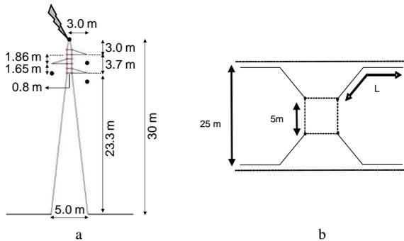
Fig. 3. Representation of the tower configurations of the 138-kV line (a) and the tower-footing arrangement consisting of counterpoise-wires of length  $L$  buried 0.5 m deep in the soil (radius of 0.75 cm) and vertical rods (3 m long and radius of 5 cm) to represent the buried metallic components of the tower.
