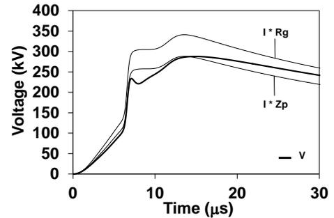
Fig. 2. Comparison of the response of the tower-footing electrodes of Fig. 3 subjected to the median first-stroke current of Fig. 1 (curve V) and those obtained assuming the representation of the tower-footing by the concentrate parameters  $R_{LF}$  and  $Z_P$ . Length of counterpoise wires  $L$  of 50 m and soil resistivity of 600  $\Omega$ m.
