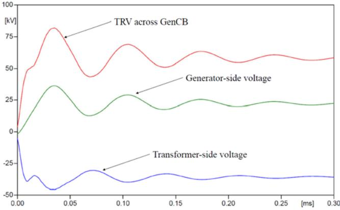
Fig. 7. Voltage waveforms in case of fault currents resulting from 180° out-of-phase conditions for the first-pole-to-clear obtained with distributed parameters models
