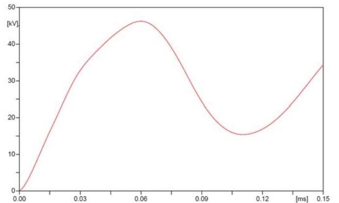
Fig. 5. TRV waveform corresponding to the first-pole-to-clear in case of a three-phase grounded fault occurring at the generator terminals
