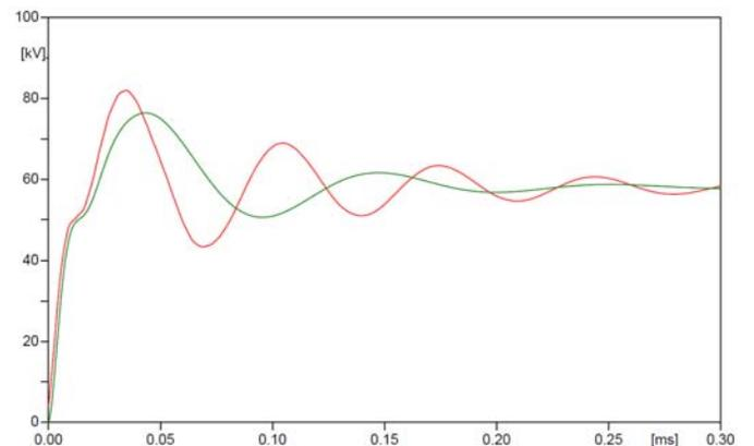
Fig. 6. TRV waveforms in case of fault currents resulting from 180° el. out-of-phase conditions for the first-pole-to-clear obtained with distributed (red curve) and lumped (green curve) parameters models
