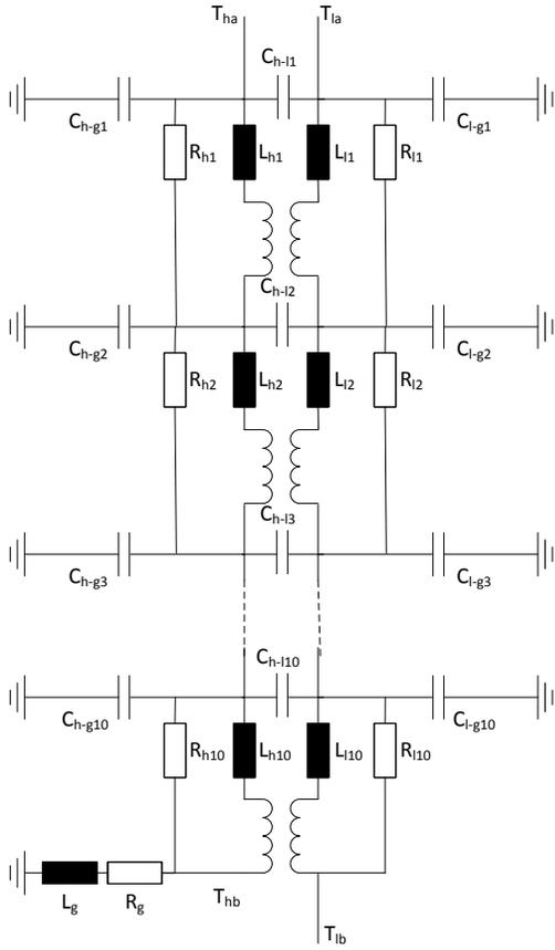
Fig. 3. Model of power transformer
