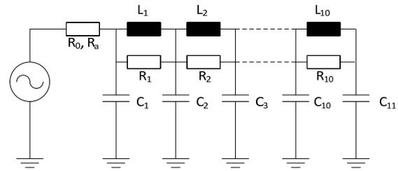
Fig. 2. Model of generator
