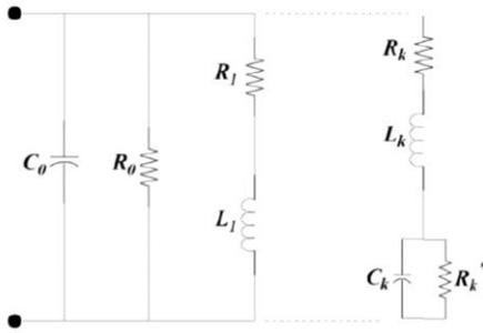
Fig. 2. Representation of the surge admittance  $Y(\omega)$  by electric circuit.
