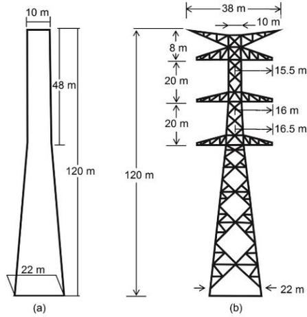
Fig. 3. Tower structure: modeled in the NEC (a) and real dimension (b).
