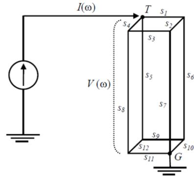
Fig. 1. Generic structure modeled as wire segments using the NEC.
