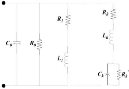
Fig. 2. Representation of the surge admittance  $Y(\omega)$  by electric circuit.
