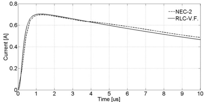
Fig. 8. Surge current through the tower simulated using the proposed model with 50 poles.
