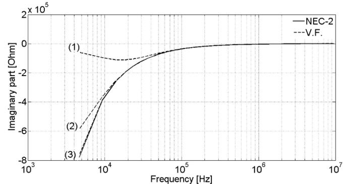
Fig. 5. Imaginary part of the surge impedance fitted with 10 (curve 1), 30 (curve 2) and 50 (curve 3) poles.
