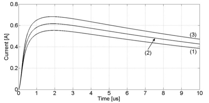
Fig. 7. Surge current through the tower simulated using the proposed time-domain model with 10 (curve 1), 30 (curve 2) and 50 (curve 3) poles.
