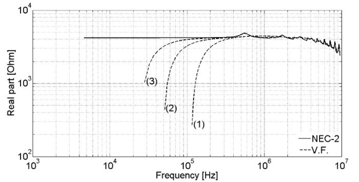
Fig. 4. Real part of the surge impedance fitted with 10 (curve 1), 30 (curve 2) and 50 (curve 3) poles.
