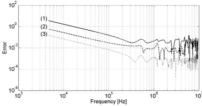
Fig. 6. Errors in the tower impedance module using the vector fitting with 10 (curve 1), 30 (curve 2) and 50 (curve 3) poles.
