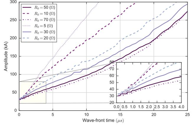
Fig. 3. Curves of limiting parameters for several different values of TL tower footing impedance.
