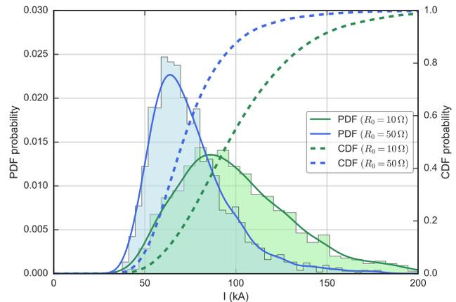
Fig. 6. PDFs and CDFs of the BF currents for two different cases of tower footing resistances.
