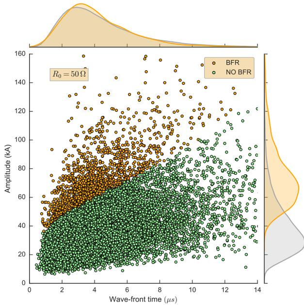
Fig. 4. Shield wire lightning currents and backflashover currents with superimposed histograms of their individual marginal distributions.
