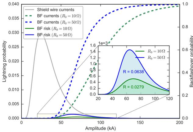
Fig. 7. Risk of backflashover computed from the shield wire incident lightning and BF lightning currents probability distributions.
