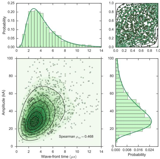
Fig. 2. Bivariate probability distribution of lightning-currents incident to TL shield wire(s) obtained with EGM according to Brown and Whitehead.
