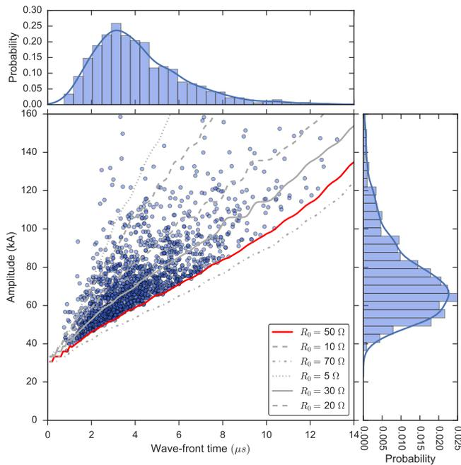
Fig. 5. Backflashover lightning currents with superimposed histograms of their marginal distributions.
