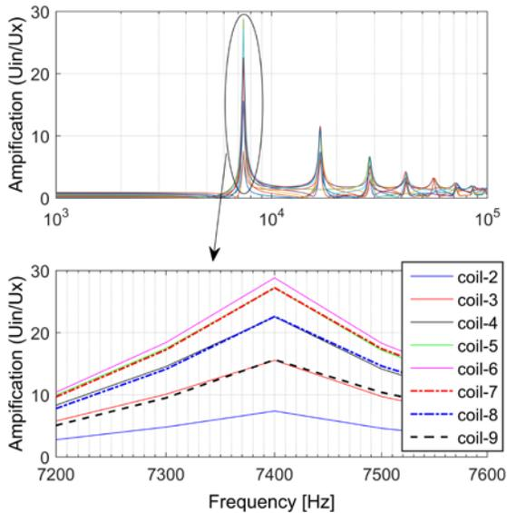
Figure 3. Computed amplification factors for all coils for the observed frequency spectrum (upper graph); increased time scale of the amplification factors around resonance frequency of 7.4 kHz.
