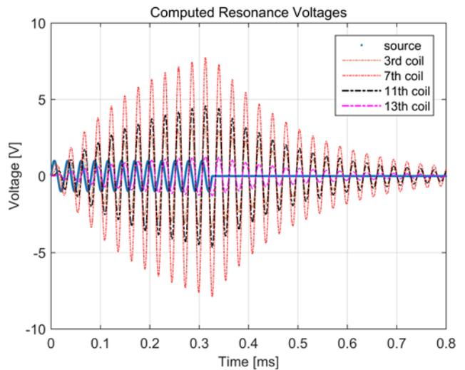
Figure 11. Computed resonance voltages for an excitation with 12 periods.
