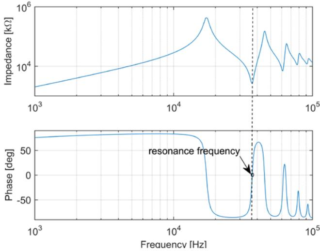
Figure 6. Harmonic terminal impedance of the studied transformer winding with the most severe resonance frequency; amplitude characteristic (upper trace) and phase characteristic (lower trace).
