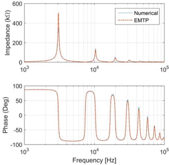
Figure 2. Comparison between numerical computation and simulation of harmonic terminal amplitude impedance (upper graph) and phase impedance (lower graph).
