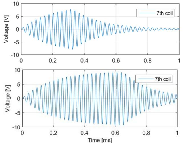
Figure I. Resonance voltage in the 7<sup>th</sup> coil for a source with 12 periods (upper graph and 24 periods (lower graph).
