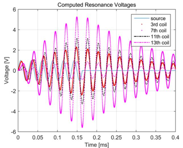
Figure 10. Computed resonance voltages for an excitation with 6 periods.
