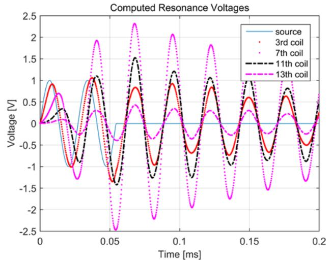
Figure 9. Computed resonance voltages for an excitation with 2 periods.
