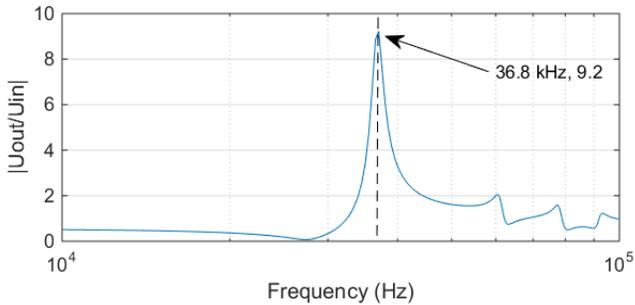
Figure 8. Computed amplification factor for coil 7.
