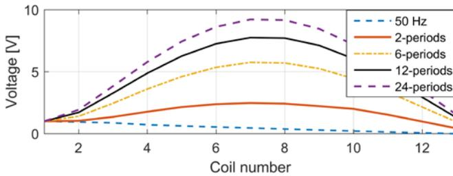
Figure 12. Voltage distribution during resonance for different duration of the excitation compared with to voltage distribution during normal operation (50 Hz).
