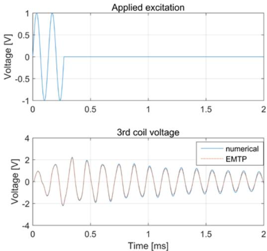
Figure 4. Applied excitation and voltage response in the 3<sup>rd</sup> coil.
