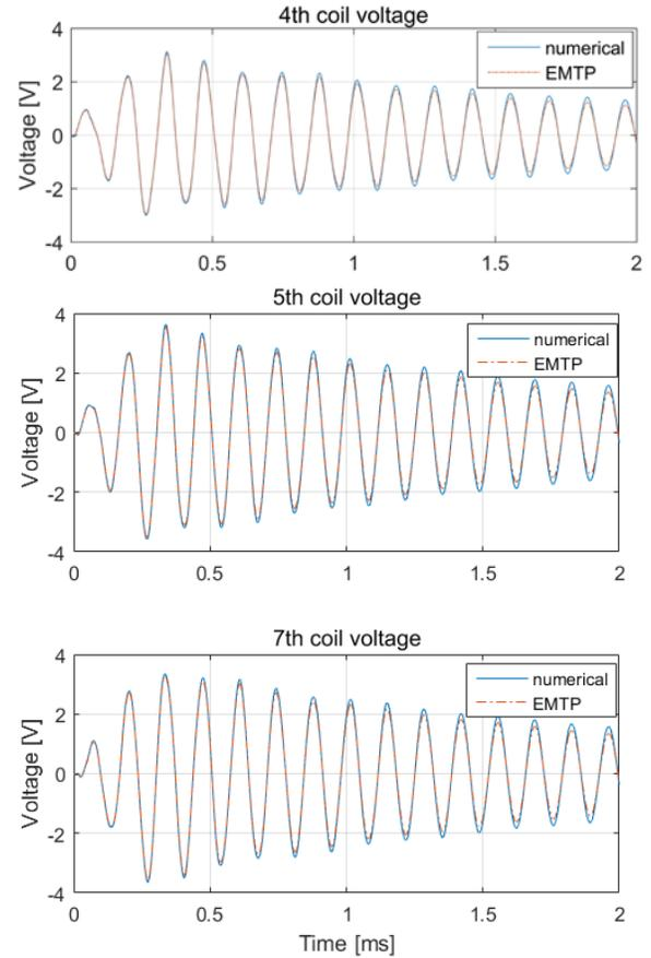
Figure 5. Voltage oscillation in coils 4, 5 and 7 upon an excitation as shown in Figure 4.
