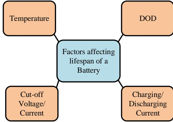
Fig. 1. Factors that affect the lifespan of a BESS-battery.
