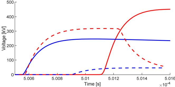
Fig. 1. Voltage in cable (blue) and OHL (red) close to the transition point. Solid lines: wave propagating from cable to OHL; Dashed lines: wave propagating from OHL to cable;
