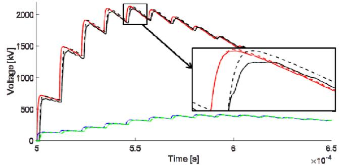
Fig. 4. Voltage at the closest OHL-cable transition for a lightning current of 24kA. Red: Lightning at 25m; Black: Lightning at 375m; Green and Blue: Voltage at sound phase; Dashed line: Without corona; Solid line: With corona
