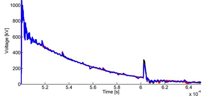
Fig. 12. Voltage in one phase at the sending end of the cable for different cable bondings for a 9000m cable. Black: Both-ends bonding; Red: 1 major cross-section; Blue: 2 major cross-sections
