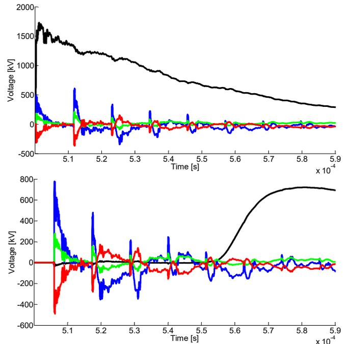
Fig. 8. Voltage propagation modes for a back flashover. Black: Ground mode; Blue, Red and Green: Coaxial modes; Up: Voltage at the cable's sending end; Bottom: Voltage at the cable's receiving end
