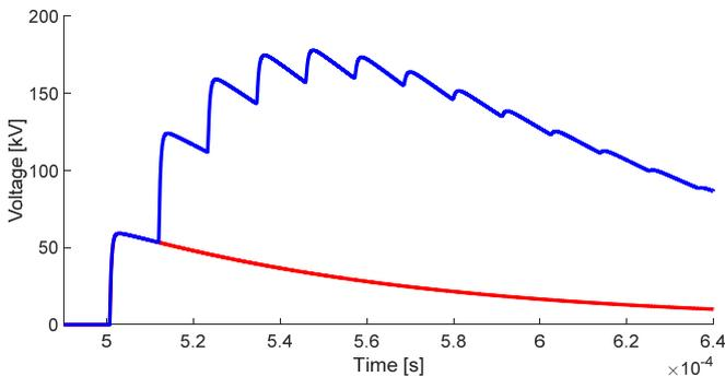
Fig. 2. Voltage at the transition point due to lightning hitting the OHL at 200m. Red: 100km long cable; Blue: 1km long cable
