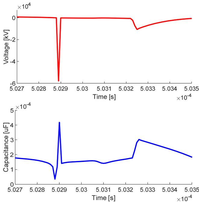
Fig. 7. Voltage (up) and capacitance value of one shunt element (down) during a transient due to lightning
