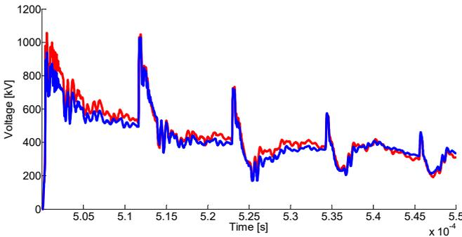
Fig. 10. Voltage in one phase at the sending end of the cable. Red: Current depending grounding only at towers; Blue: Current depending grounding at towers and screen's grounding points
