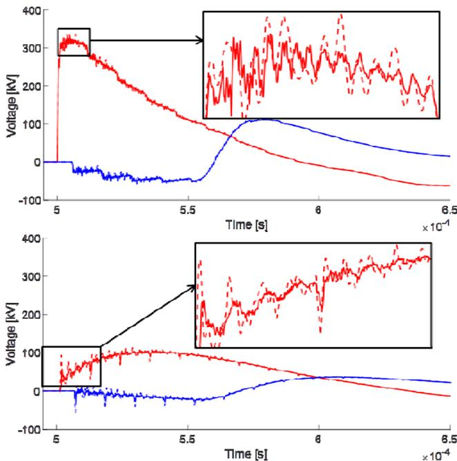
Fig. 5. Voltage in one phase at the sending (Red) and receiving (blue) ends of the cable. Solid lines: With corona; Dashed lines: Without corona; Up: Lightning at 25m; Down: Lightning at 375m
