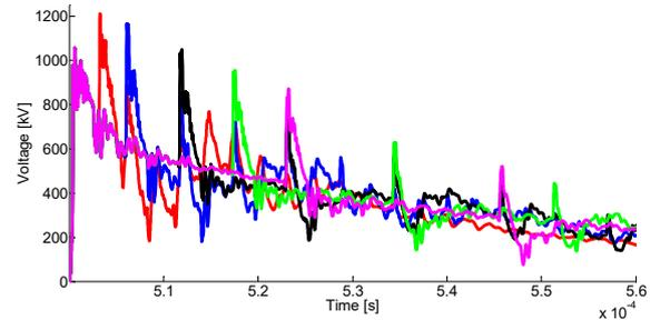
Fig. 11. Voltage in one phase at the sending end of the cable for different cable lengths. Red: 250m; Blue: 500m; Black: 1000m; Green: 1500m; Magenta: 2000m
