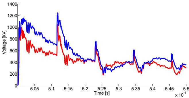
Fig. 9. Voltage in one phase at the sending end of the cable. Red: Current depending grounding at towers; Blue: Fixed  $20\Omega$  grounding
