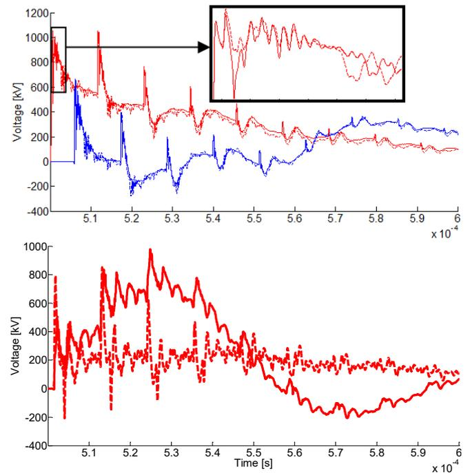
Fig. 6. Voltage in one phase at the sending (Red) and receiving (blue) ends of the cable. Solid lines: With corona; Dashed lines: Without corona; Up: Lightning at 25m; Down: Lightning at 375m
