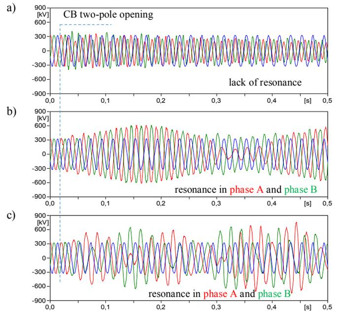
Fig. 8. EMTF-ATP simulation, two-pole opening of shunt reactor and OHL; various combinations: a) OHL 2, b) OHLs 1+3, c) OHLs 1+2+3
