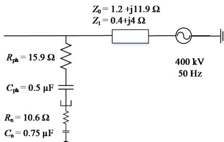
Fig. 4. Frequency dependent network equivalent diagram
