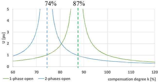
Fig. 5. Induced voltages with respect to compensation degree  $k$
