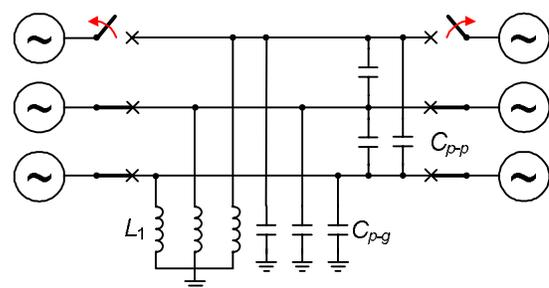
Fig. 1. General diagram for single-phase opening of OHL and shunt reactor:  $L_1$  – main shunt reactor's inductance,  $L_N$  – NGR's inductance,  $C_{p-g}$  – phase-to-ground capacitance of the OHL,  $C_{p-p}$  – phase-to-phase capacitance of the OHL
