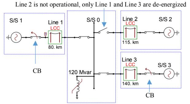
Fig. 6. Example of network configuration leading to resonance (OHLs 1+3)
