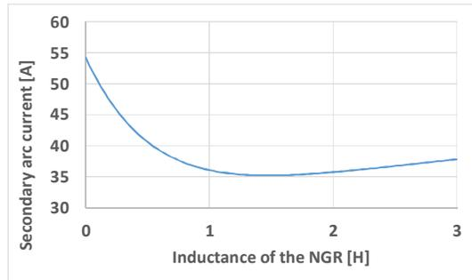
Fig. 10. Secondary arc current in the function of NGR's inductance with main shunt reactor rated at 120 Mvar
