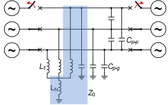
Fig. 2. De-energization of the faulted phase, NGR installed,  $L_1$  – main shunt reactor's inductance,  $L_N$  – NGR's inductance,  $C_{p-g}$  – phase-to-ground capacitance of the OHL,  $C_{p-p}$  – phase-to-phase capacitance of the OHL,  $Z_0$  – equivalent zero sequence impedance
