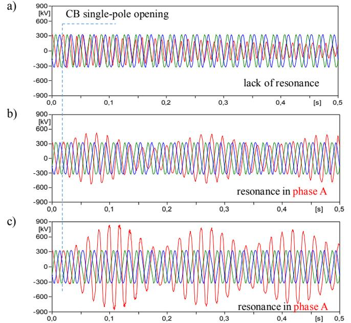
Fig. 7. EMTF-ATP simulation, single-pole opening of shunt reactor and OHL; various combinations: a) OHL 2, b) OHLs 1+3, c) OHLs 1+2+3
