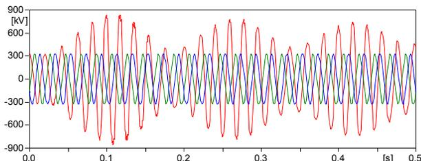
Fig. 9. EMTP-ATP simulation, single-pole opening at  $t = 20$  ms of shunt reactor and OHLs 1+2+3, Cassie-Mayr model used for CB modelling
