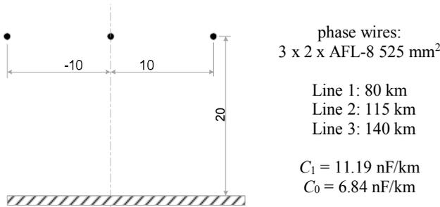
Fig. 4. Overhead line layout and phase wire's data
