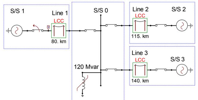
Fig. 3. Simplified general layout of the studied 400 kV network
