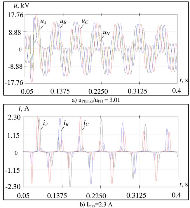
Fig. 4. Calculated oscillograms of phase voltages (a) and VT primary currents (b) during stable group ferroresonance in the 6 kV industrial network with ungrounded neutral ( $I_C = 13.4$  A, 8 VTs)
