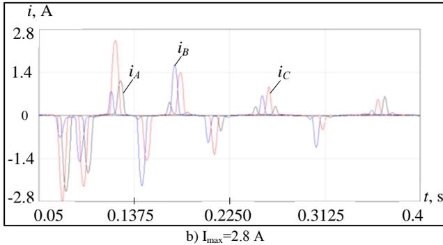
Fig. 5. Calculated oscillograms of phase voltages (a) and VT primary currents (b) during unstable group ferroresonance in the 6 kV industrial network with ungrounded neutral ( $I_C = 24.7$  A, 10 VTs)
