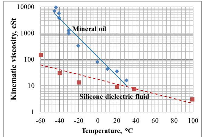
Fig. 7. Measured values of kinematic viscosity for mineral oil and silicone dielectric fluid
