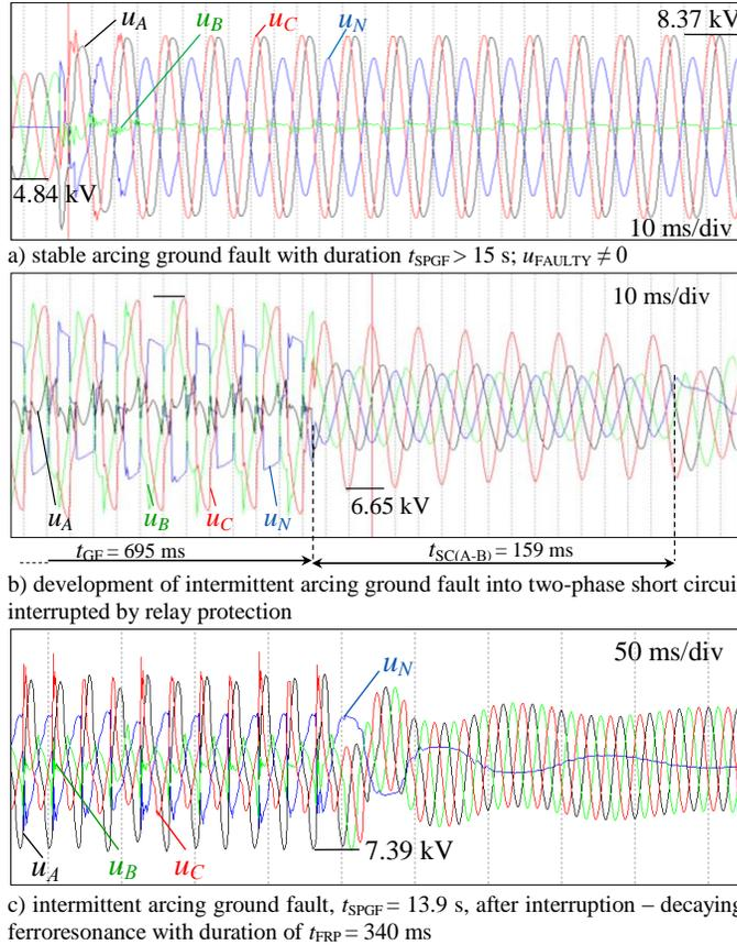
Fig. 2. Real oscillograms of phase voltages at arcing ground faults in the 6 kV cable network with ungrounded neutral,  $I_{SPGF 50 Hz} = 12 - 14$  A
