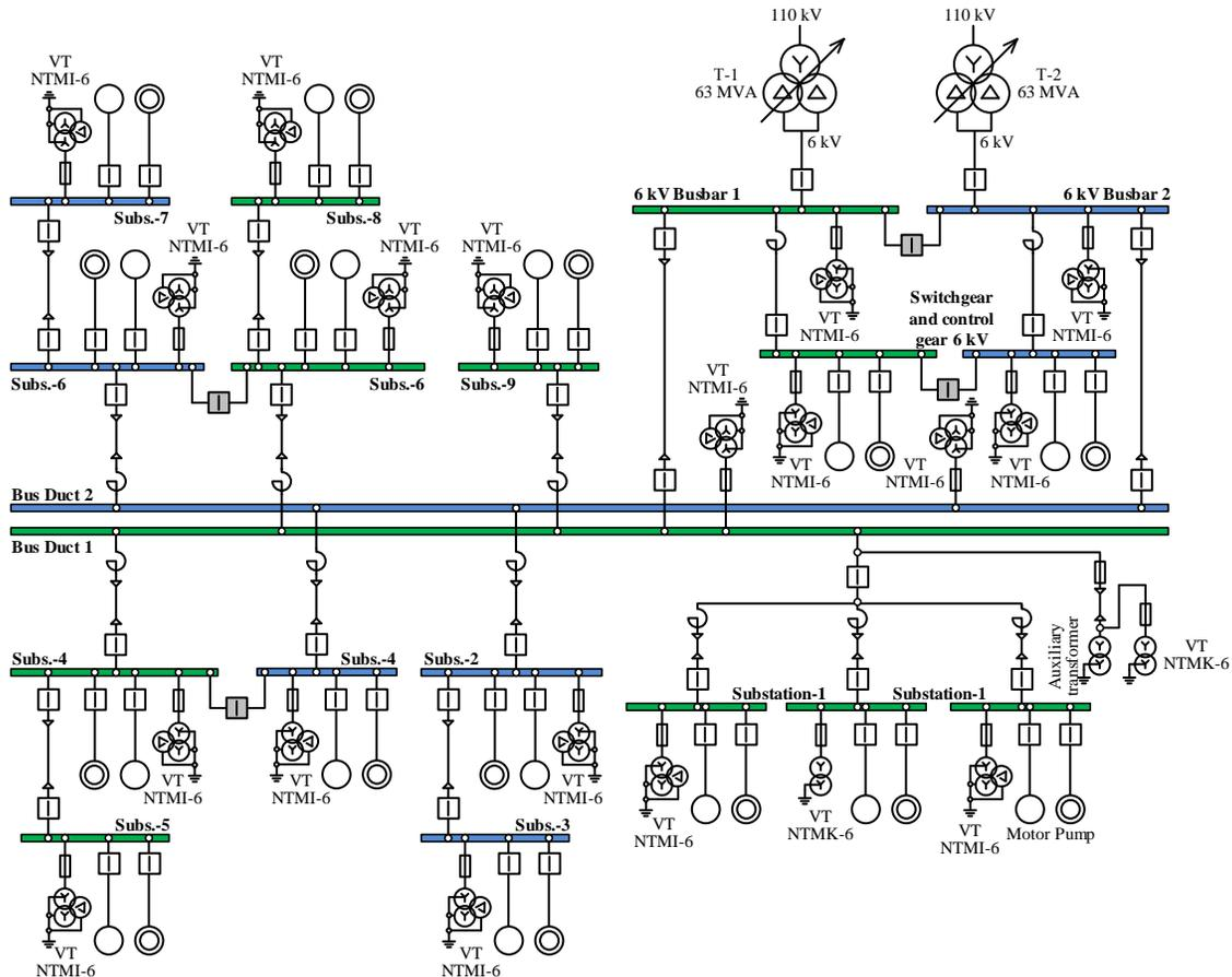
Fig. 1. Simplified single-line diagram of the first primary substation
