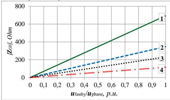
Fig. 3. Engineering assessment of a ground fault impedance at insulation breakdown during a stable arcing ground fault in the 6 kV network with different capacitive currents: 5 A (curve 1), 10 A (curve 2), 15 A (curve 3), 30 A (curve 4)
