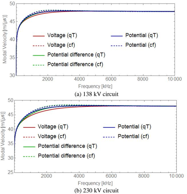
Fig. 4. Ground mode velocity for the two test cases line considering the three distinct formulations.
