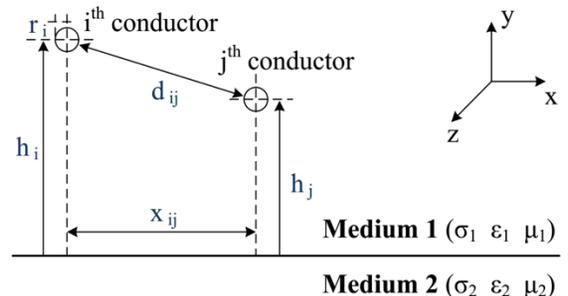
Fig. 1. Configuration of the conductors for an overhead line
