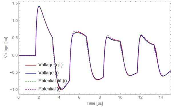
Fig. 13. Voltage response at node #6 for the 230 kV line.
