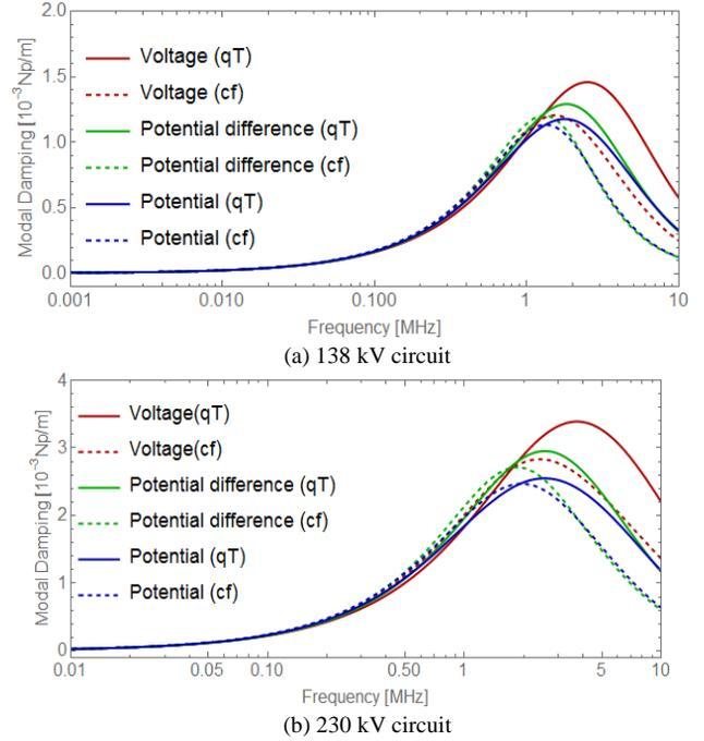
Fig. 3. Ground mode damping for the two test cases considering the three distinct formulations.
