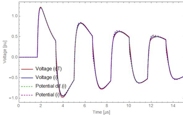
Fig. 11. Voltage response at node #4 for the 138 kV line.
