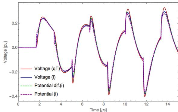
Fig. 12. Voltage response at node #6 for the 138 kV line.
