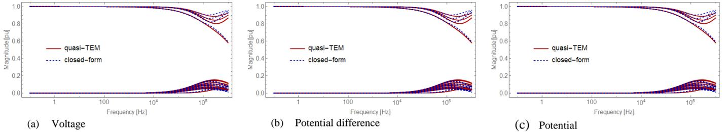
Fig. 7. Propagation function for the 138 kV line considering the three distinct formulations.
