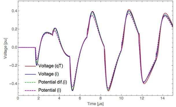
Fig. 14. Voltage response at node #6 for the 230 kV line.
