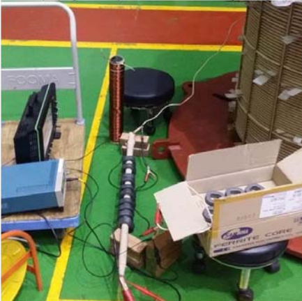
Fig.8. Laboratory test set-up with ferrite rings and Ayrton-Perry winding for preliminary low-voltage comparison of VFTO damping effectiveness.
