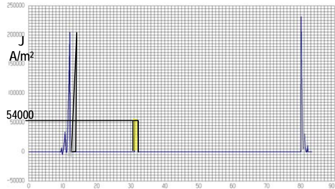
Fig. 3b. Current density J(R) distribution in VFTO damping section of GIS at 1 MHz. Values read from the graph confirm analog calculations:
