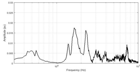
Fig. 15. FFT of the maximum voltage impulse from the switching operation— Measurement.
