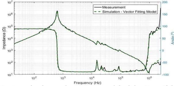
Fig. 5. Comparison between the measurement and simulation: Vector Fitting model.
