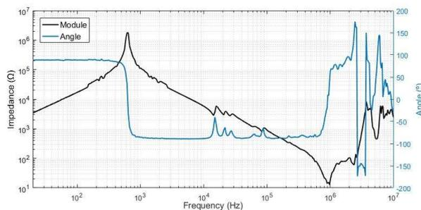
Fig. 2. Measurement of impedance along the frequency range seen at the high voltage terminal.
