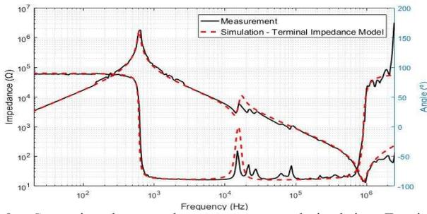
Fig. 9. Comparison between the measurement and simulation: Terminal Impedance model.
