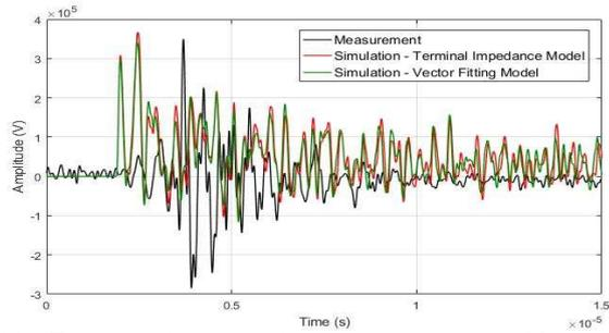
Fig. 16. Transient voltage from the switching operation – Measurement x Simulation.
