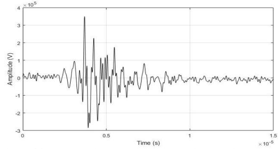
Fig. 14. Maximum voltage impulse from the switching operation—Measurement.
