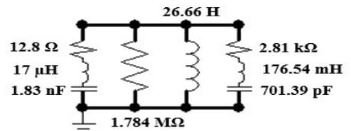
Fig. 8. Synthesized circuit: Terminal Impedance model.
