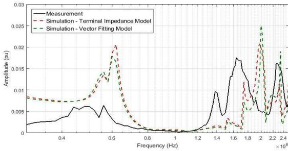
Fig. 17. FFT of the transient voltage from the switching operation – Measurement x Simulation.
