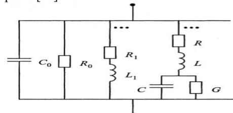
Fig. 3. Synthesized RLC circuit: using Vector Fitting [12].
