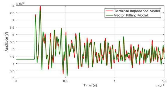
Fig. 11. Transient voltage from the switching operation - Simulation: Terminal Impedance model and Vector Fitting model.
