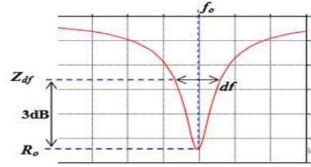
Fig. 7. Bandwidth relative to its center frequency.
