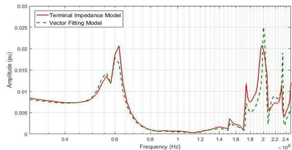
Fig. 12. FFT of the transient voltage from the switching operation - Simulation.
