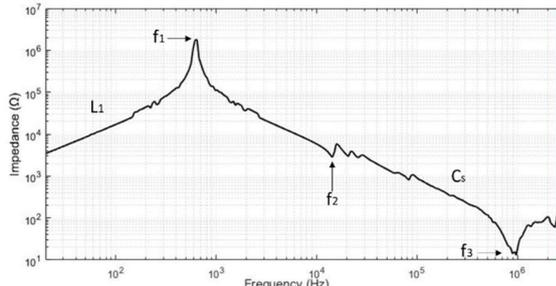
Fig. 6. Measurement of the impedance module in the frequency range seen from the high voltage terminal – Highlight for the points considered in the modeling.
