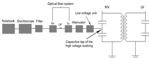
Fig. 13. Transient voltage measurement system integrated into the capacitive tap of the high voltage bushing of the power transformer.
