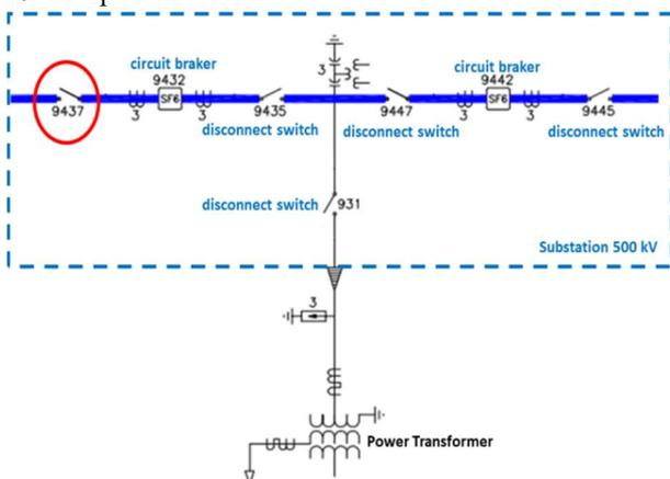
Fig. 10. Diagram of the section of the substation.
