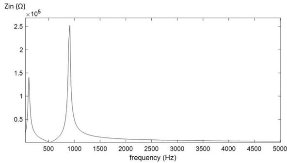
Fig. 6. Input impedance of the phase a of the system versus frequency at the HV terminal of the transformer when the transformer is loaded.
