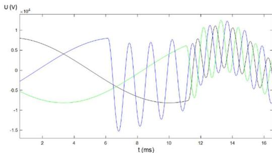
Fig. 7. Phase to ground overvoltages (V) at the HV terminals of the transformer when the restrike-free breakers are opened at 4 ms.
