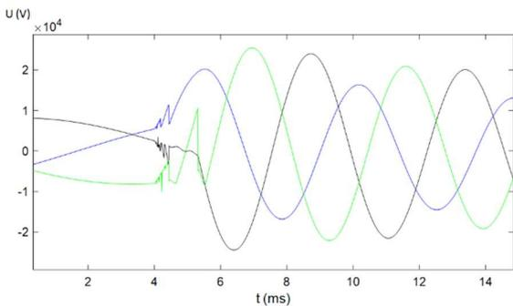
Fig. 12. Phase to ground overvoltages (V) at the transformer's MV terminals when a RC filter is placed close to the VCB
