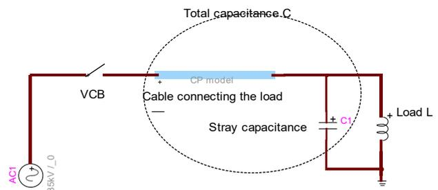
Fig. 1. Opening of an inductive load with a VCB.
