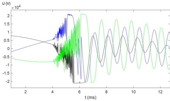
Fig. 10. Phase to ground overvoltages (V) at the transformer's terminals, after the VCBs when the arresters are installed at the source side.
