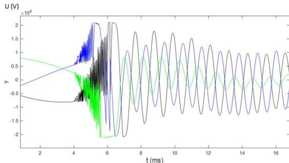
Fig. 9. Phase to ground overvoltages (V) at the source terminals, after the VCBs, when the arresters are installed at the transformer.
