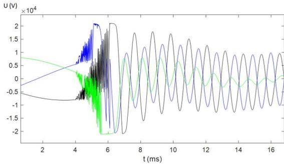
Fig. 11. Phase to ground overvoltages (V) at the source terminals, after the VCBs, when the arresters are installed at the source side.
