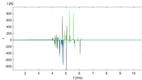
Fig. 5. Current (A) circulating in one phase of the VCB. It is constituted of a series of impulses due to the successive arc interruptions and reignitions.
