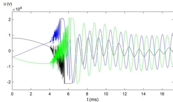
Fig. 8. Phase to ground overvoltages (V) at the transformer MV terminals when arresters are installed directly at the transformer.
