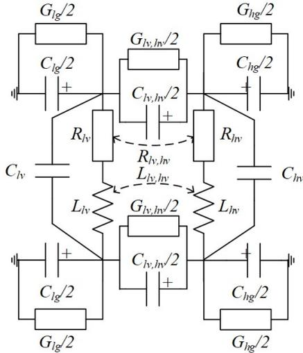
Fig. 3. RLCG network for one phase of a two-winding transformer.
