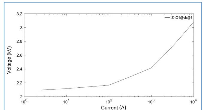
Fig. 13. Characteristic of the arrester.
