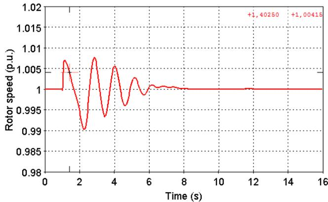
Fig. 8 Generator speed for  $b = 0.26$  pu
