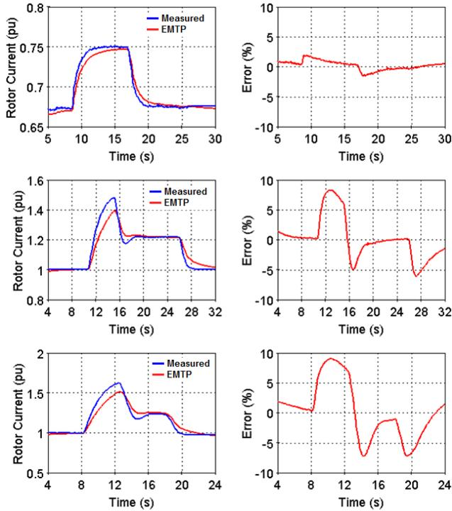
Fig. 2 Time domain rotor current  $I_f$  comparison between calculation and measurement
