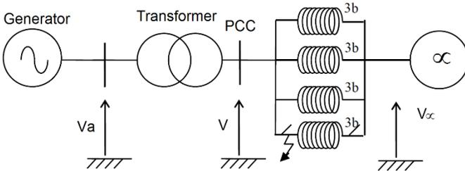
Fig. 4. Simplified circuit used for the study of stability on short circuit [4]
