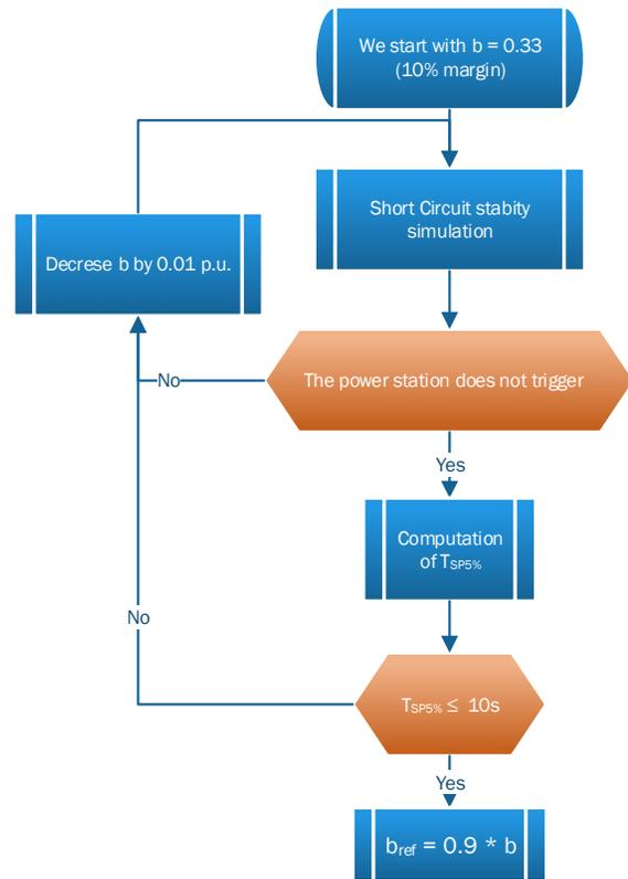
Fig. 5 Iterative method in order to determine the  $b$  reactance and  $T_{SP5\%}$
