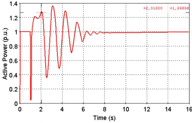
Fig. 6 Active power at PCC for  $b = 0.26$  pu
