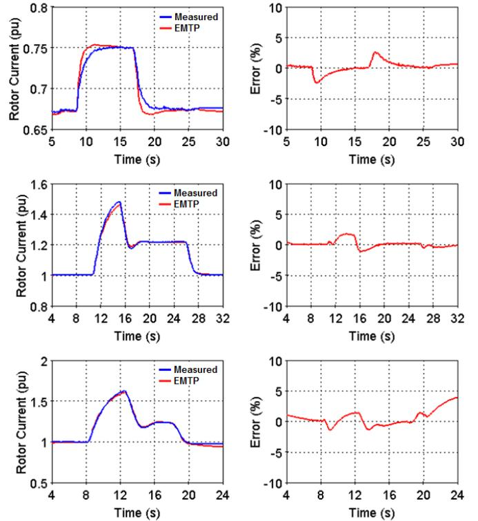
Fig. 3 Time domain rotor current  $I_f$  comparison between calculation and measurement after the model calibration
