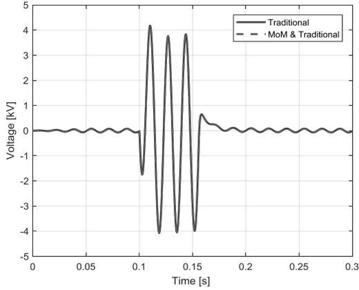
Figure 4. Induced voltage on aerial pipe
