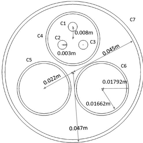
Figure 5. Non-conventional pipe-type cable example
