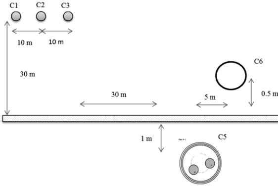
Figure 1. Transmission line configuration with overhead lines and cables
