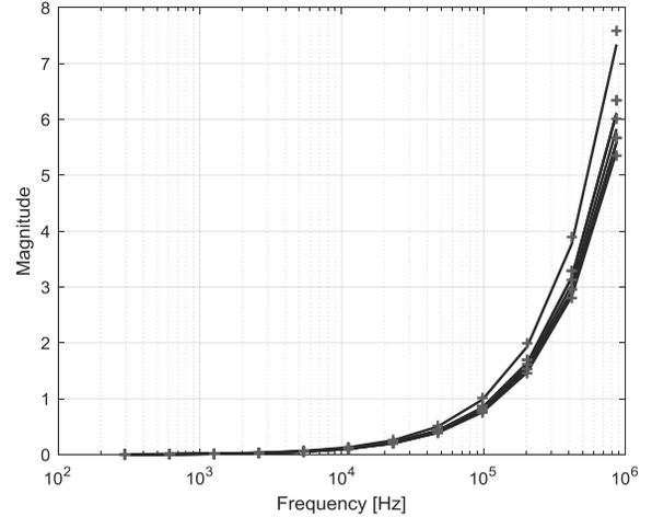
Figure 6. Magnitude of first column of impedance matrix ('+' curve – proposed method, solid curve – MoM method)
