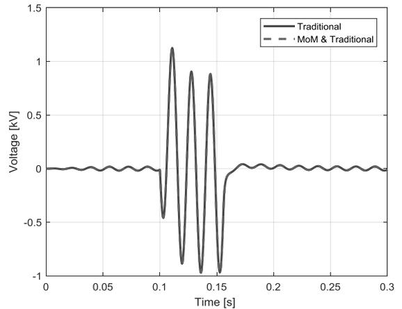
Figure 3. Induced voltage on underground pipe of the pipe-type cable
