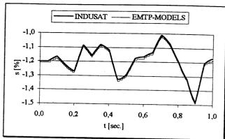
Figure 6: Comparison between INDUSAT and EMTP results (induction generator slip).
