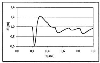
Figure 11: Loss of load, field voltage, AVR operation.
