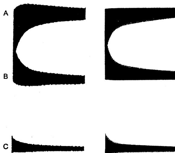
Figure 6. Damping of the measured (curves in the left) and simulated (curves in the right) inrush currents of phases A, B and C in six seconds.
