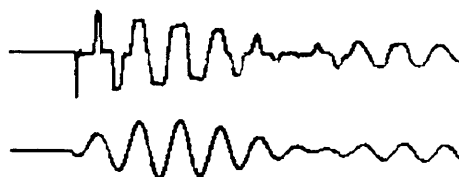
Voltage in phase b (point B) upper curve: real network lower curve: reference network
