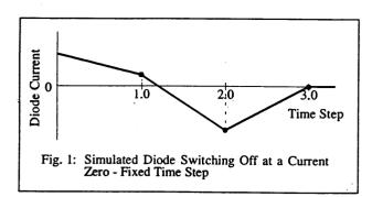
A smaller time step can be used to minimize these errors, but will result in longer execution times. A multiple or variable time step algorithm can also be applied, but requires significant structural changes to existing programs and will result in longer execution times.
