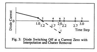
This interpolation method is nearly transparent to all other controls and system models and can thus be implemented in existing programs without major compatibility problems. An enhancement of the method described above which allows instantaneous transitions due to switching operations as opposed to transitions which occur over one time step, is presently being tested.
