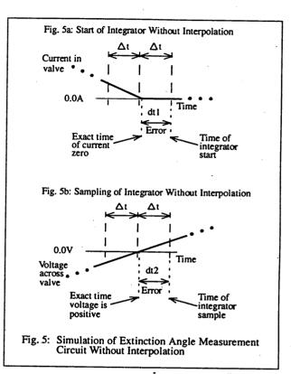
In order to implement linear interpolation within this circuit, it is necessary to calculate correction factors at both the time step of starting the integrator and at sampling of its output. With reference to Fig. 5a, the correction factor required at the time step of starting the integrator corresponds to the output of the integrator over time dt1 and is given by:
