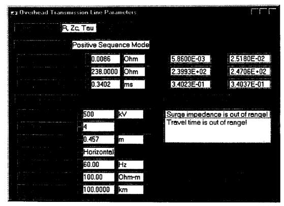
Fig. 1. User Interface for Data Validation for Positive Sequence Mode of OHL
