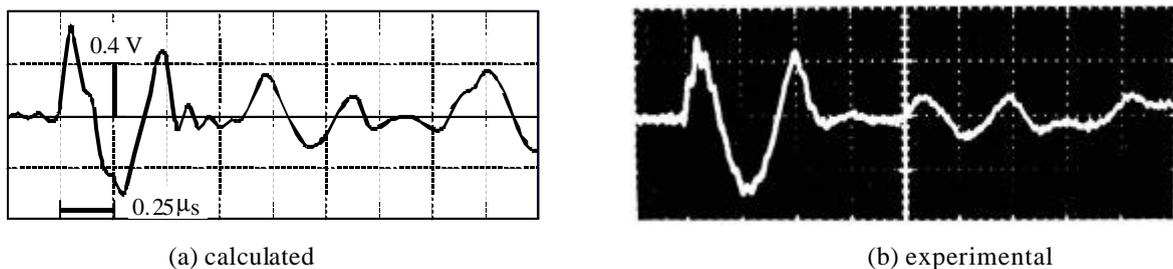
Fig. 11. Voltage induced at first interturn  $\delta v_1$  of 500 kV autotransformer subjected to sinusoidal pulse.
