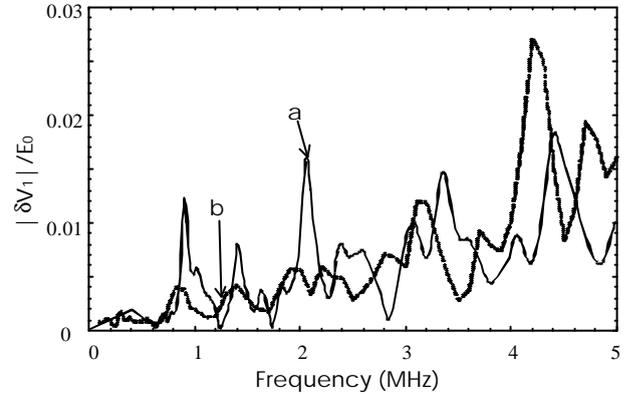
Fig. 8 Frequency characteristics of first interturn voltage of 500kV autotransformer..
