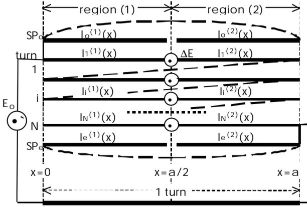
Fig. 2. MTL model of shell-form transformer.
