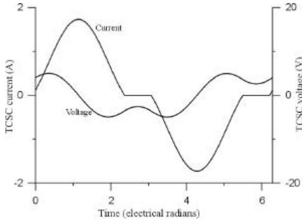
Fig. 11 – ASC voltage and the reactor current ( $\sigma=140^\circ$ )
