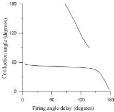
Fig. 6 – Conduction angle of single-phase Static VAR Compensator
