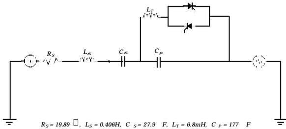
Fig. 2 – Kayenta Advanced Series Compensator
