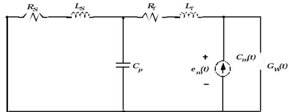
Fig. 5 – Small-signal equivalent circuit of single-phase Static VAR System
