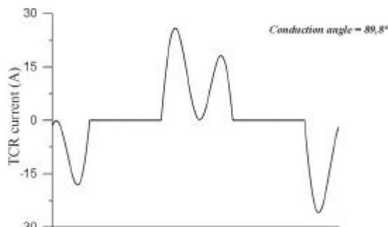
Fig. 8 – Steady-state reactor current
