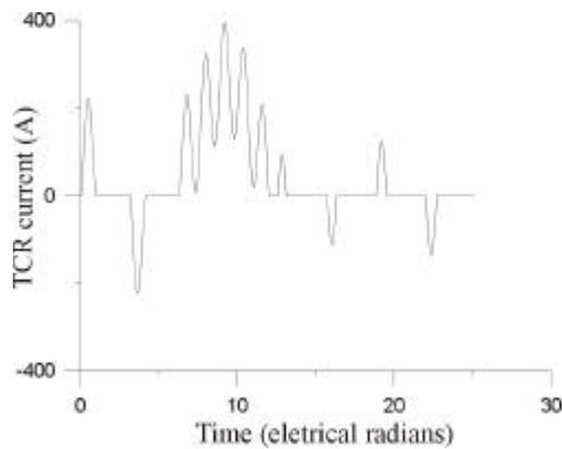
Fig. 7 – Reactor current transient
