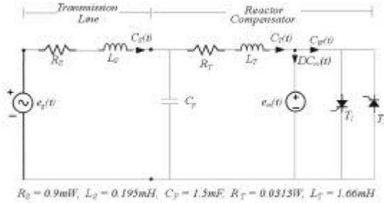
Fig. 1 – Single-phase Static VAR System
