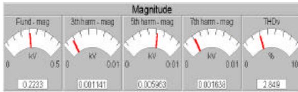
Fig. 12. Harmonic Voltages on bus 19 LV
