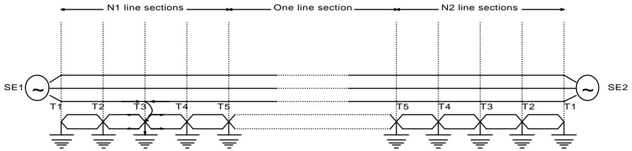
Figure 3 – Diagram showing the modeling of the transmission line
