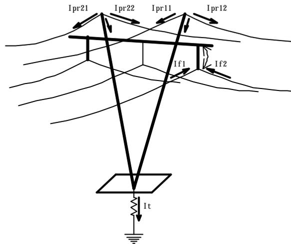
Figure 2 – Circulation of fault currents in the cables and in the ground
