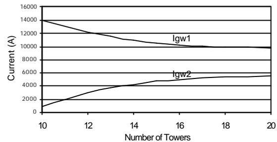
Figure 5 – Currents in the ground wires
