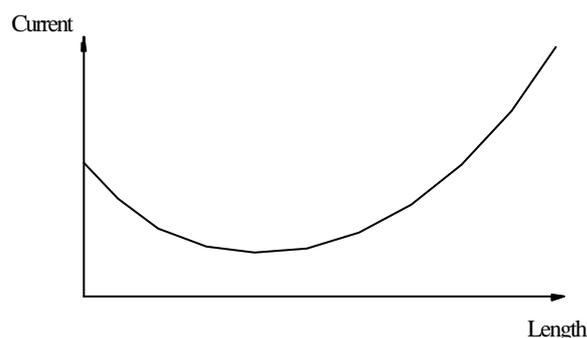
Figure 1 – Variation of the fault current along the transmission line
