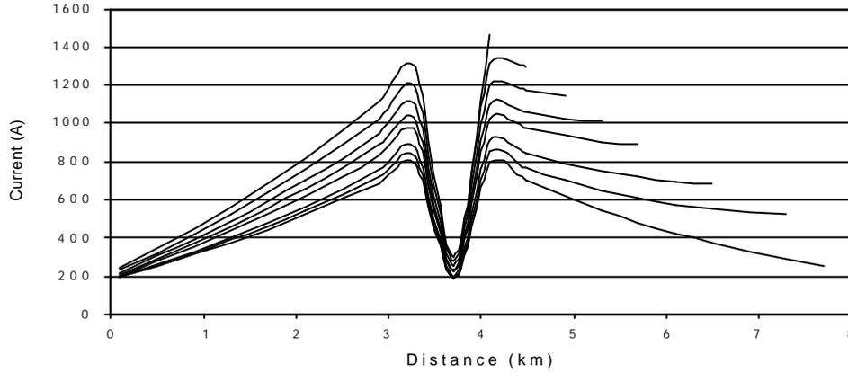
Figure 4 - Currents in the tower-footing resistances
