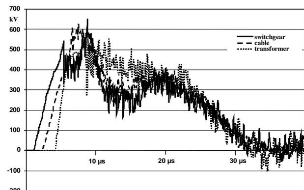
Fig. 9. Lightning voltage stresses following a direct strike to the overhead line conductor in the vicinity of tower 1
