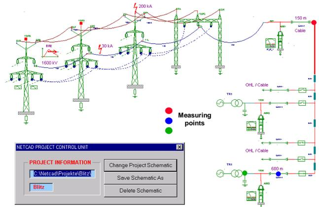
Fig. 8. Example for a lightning study of a 230 kV GIS
