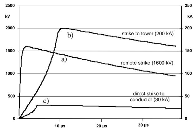
Fig. 1. Simulation of lightning currents and voltages
