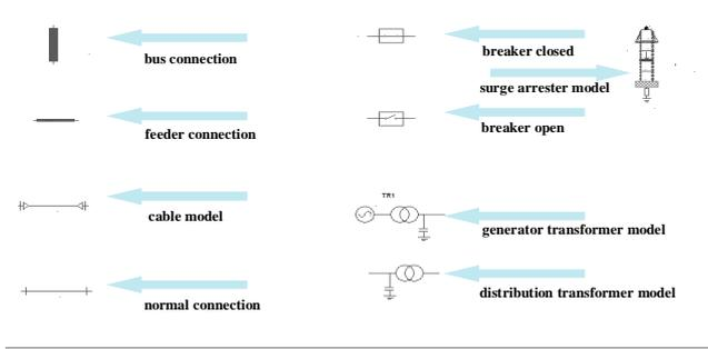
Fig. 6. Models for switch gear components
