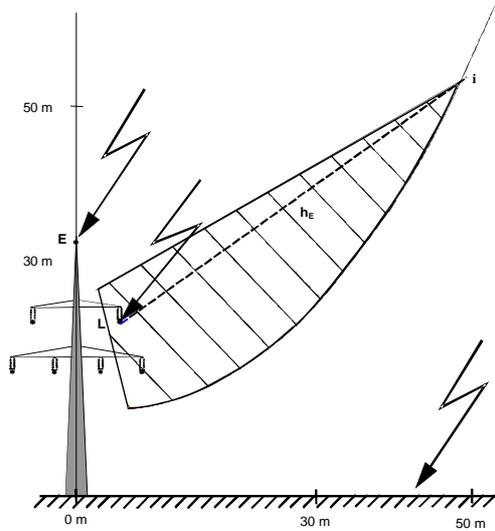
Fig. 2. Electrogeometric model of a tower to calculate maximum direct lightning strikes
