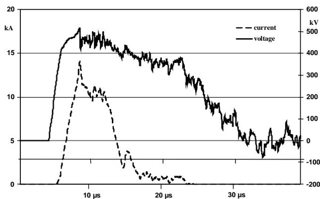
Fig. 10. Current and voltage applied at transformer arrester
