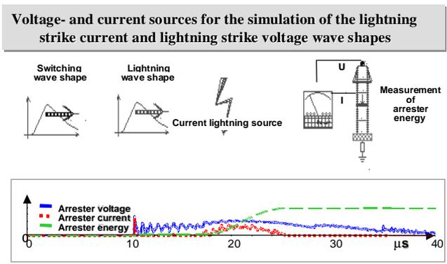
Fig. 7. Voltage- and current sources used to simulate lightning phenomena
