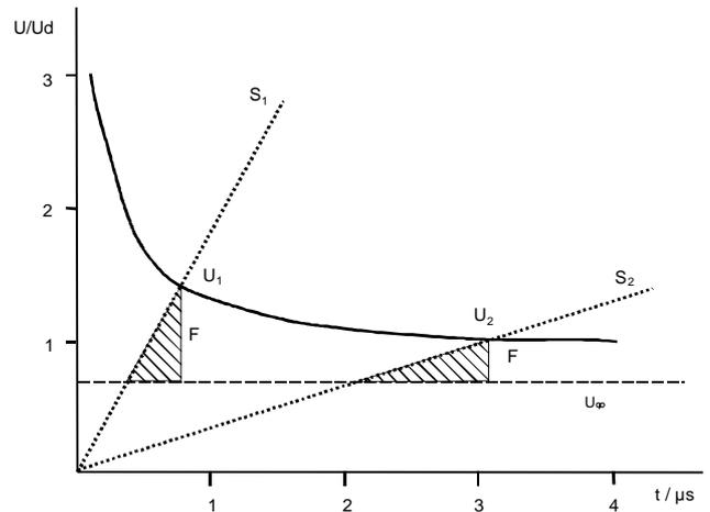
Fig. 3. Sparkover voltage versus time of an insulator
